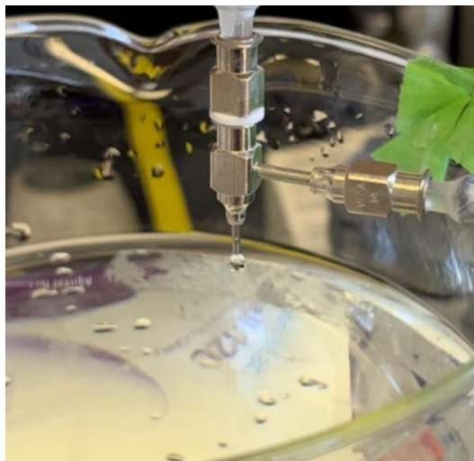
Fig. 25. Formation of CA “droplets”. Bore rate = 1.7 mL/min, dope rate = 0.67 mL/min.
