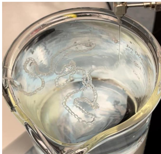
Fig. 28. Formation of CA HFs. Bore rate = 10.3 mL/min, dope rate = 4.1 mL/min.
