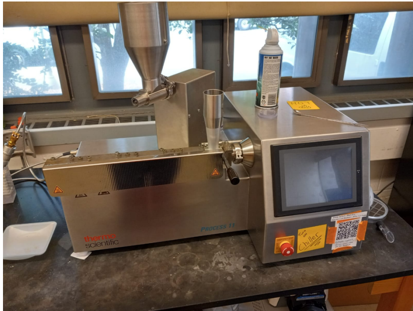
Figure 7. The extruder that was used to homogenize the spirulina and sorbitol powders.
