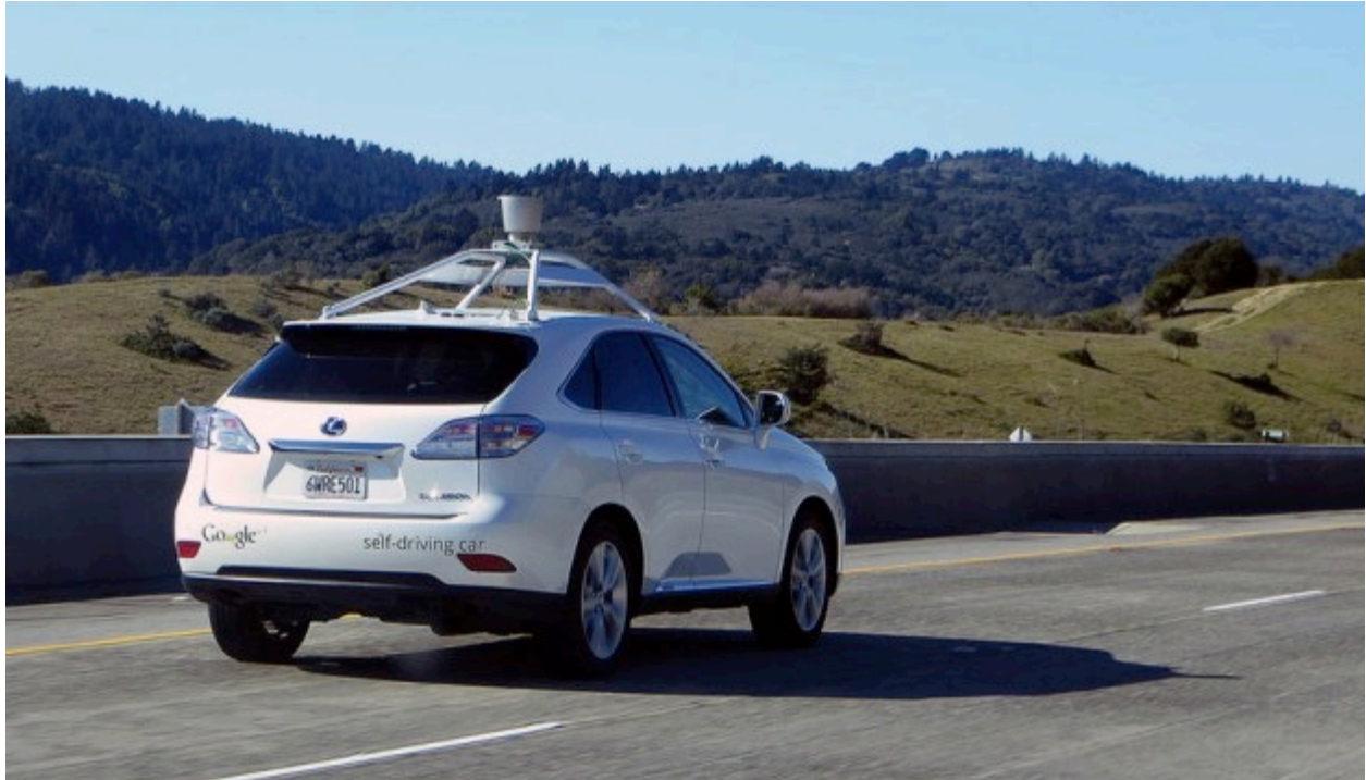
Figure 1: Google Testing Vehicle – Lexus RX450h with LIDAR sensor 3
