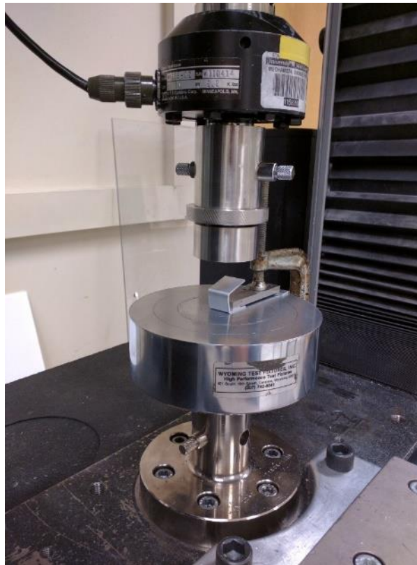
Figure 5.7. The armature is clamped to the base as the force transducer is jogging down.
