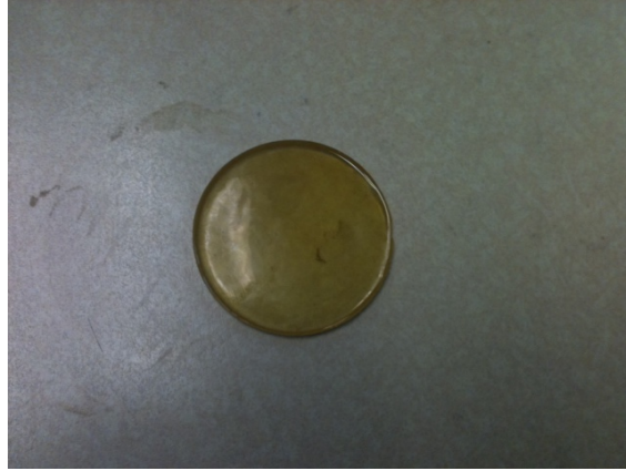
Figure V-58 Crosslinked SMP-10 under vacuum and at 400°C
