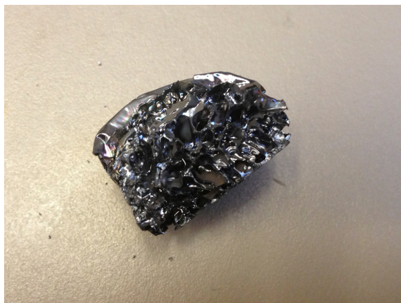
Figure V-17 1 wt% decaborane in SMP-10
