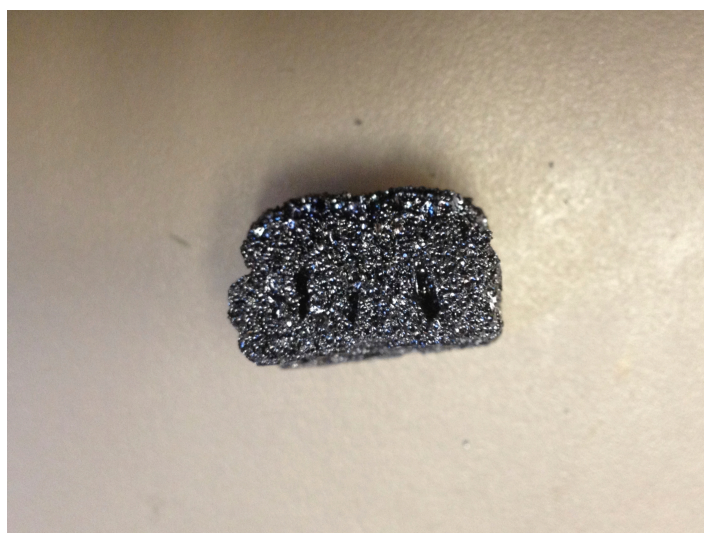
Figure V-16 Foaming with ADA alone and the presence of gaps within
