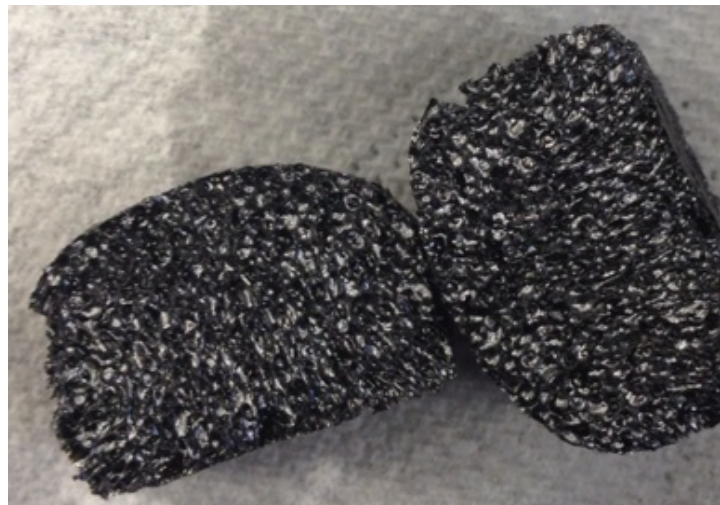
Figure V-23 Foamed SiC Monolith
