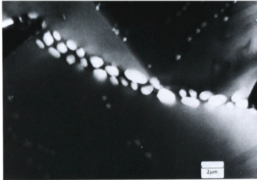
Figure II-1 Helium accumulation at the grain boundaries 10
