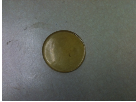
Figure V-66 Curing at 1°C/min (SMP-10 w/ 1 wt% dicumyl peroxide)
