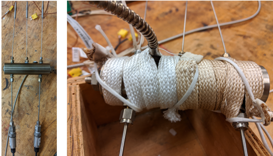
Figure 3.9: Laboratory thruster without (left) and with (right) heat tape. The color change in the heat tape is due to one having been used before. The three thermocouples extend from the top of the thruster and the two pressure transducers from the bottom, with an additional thermocouple tapped to the surface.
