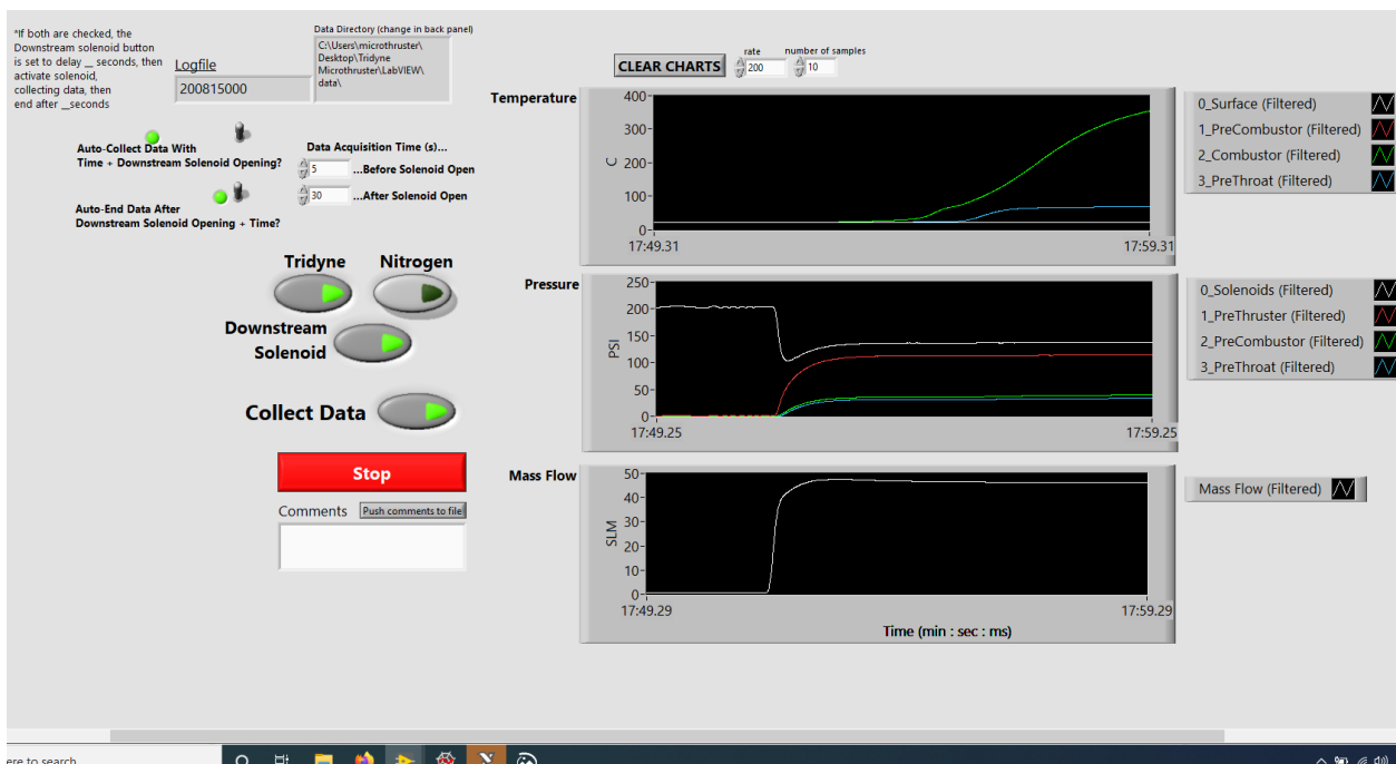
Figure 3.12: LabVIEW graphical user interface to control the bench-top thruster experiment. Back-end of LabVIEW code is available .
