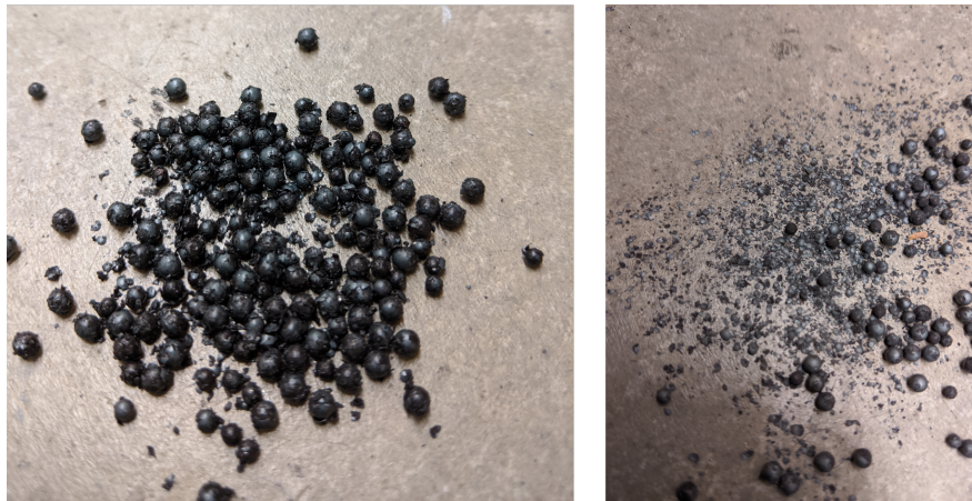
Figure 4.5: Broken down chrome steel balls after extended heating above 1100 K. Left, slag attached to balls after immediately leaving the thruster. Right, residue dislodged from the balls by manually rolling on a surface.
