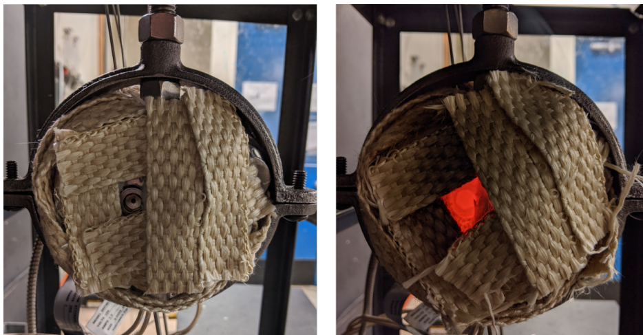
Figure 3.8: Laboratory insulated thruster without heat (left, 20^{\circ}\text{C} ) and with heat (right, 850^{\circ}\text{C} ). The strong red glow for the heated case is due to black body radiation for hot steel.
