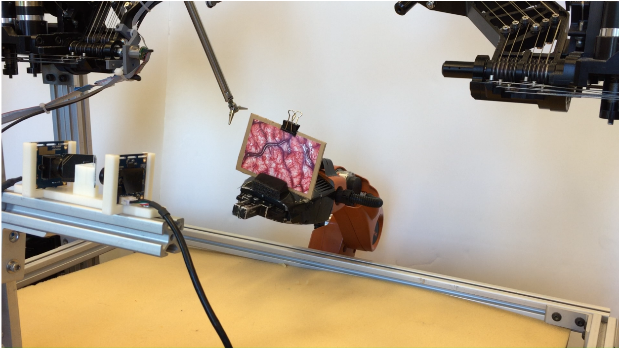
Figure 3.1: Test setup used during the testing procedure with a Kuka youBot arm holding a tissue surface within the workspace of both the RAVEN and reduced-baseline stereo camera.
