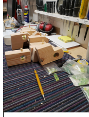
Fig 1.2 Pictured above: Figure 1.2 displays some of the buildings that will be used, note the level device embedded inside each building block.
