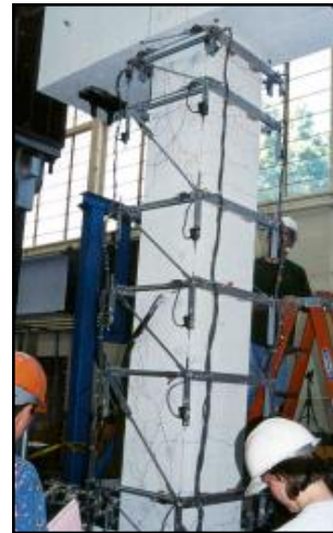
Figure 3.23 (S1 & S2) Flexural and Shear Cracking
