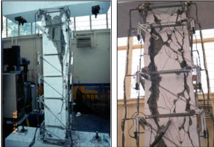
Figures 3.78 and 3.79 Concrete spalling on side faces: experimental damage (Sezen 2002)
