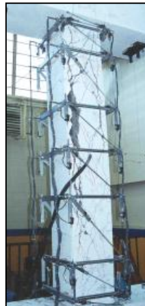
Figures 3.25 and 3.26 (S3.2) Concrete Spalling on Side Faces
