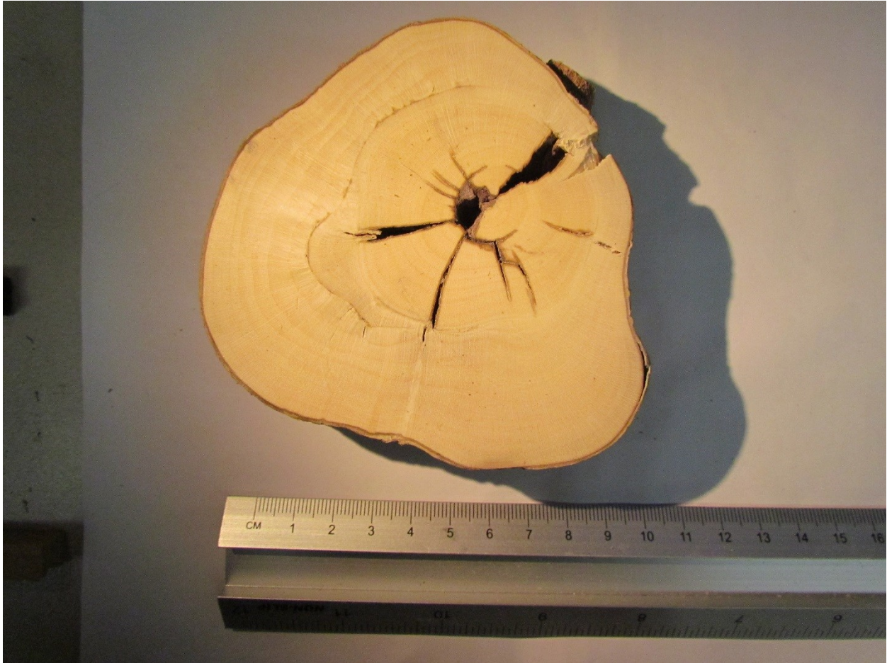
Photo 3. English holly #816, sampled as part of BAI study but not analyzed due to the large fissures shown here, which could be damaged sustained during logging operations.
