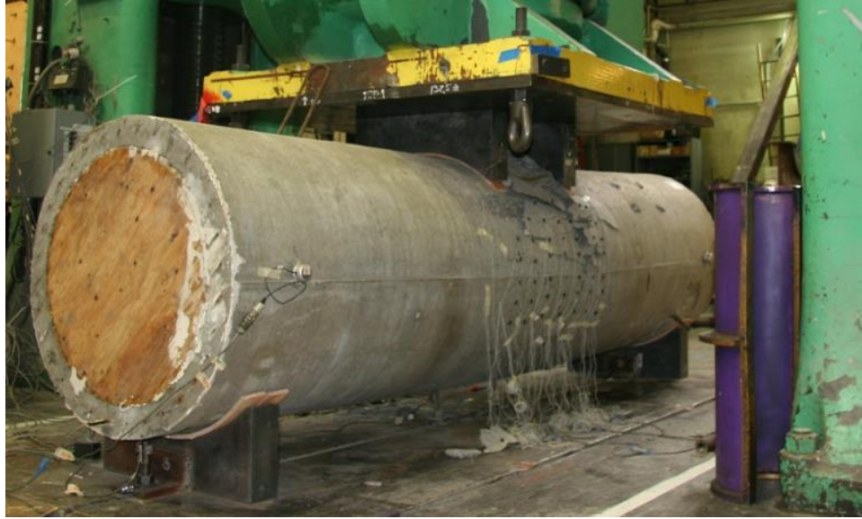
Figure 4-3. Specimen position at failure
