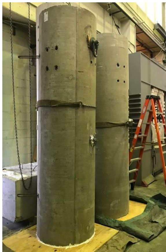
Figure 3-12. Specimen orientation prior to casting fill concrete
