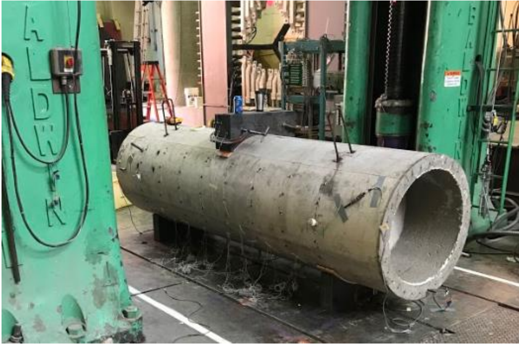
Figure 3-29. Three-point bending test optotrak and instrumentation
