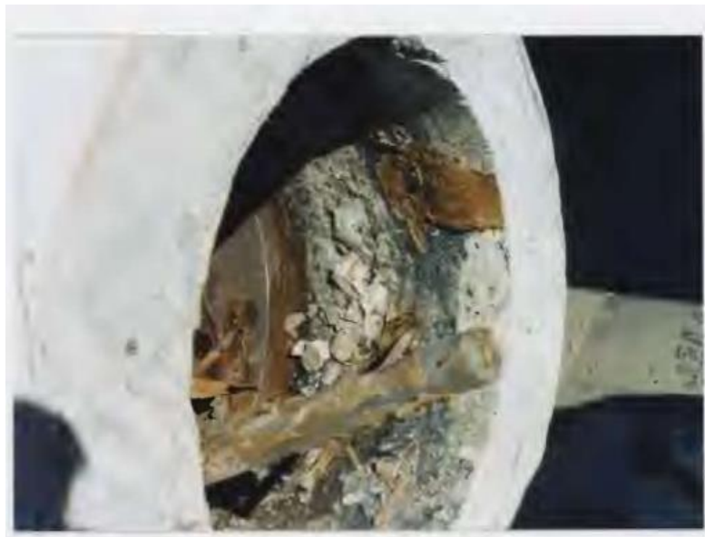
Figure 2-1. Internal spalling at core face of hollow specimen (Fig. 6.1.2., Budek, Benzoni and Priestley, 1997)
