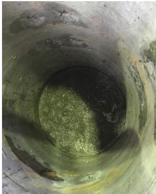
Figure 3-19. Middle diaphragm cast into Three-point bending specimen
