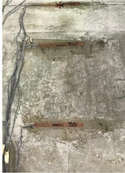
Figure 3-24. Exterior 90 mm strain gages on outer wall of Four-point bending test specimen
