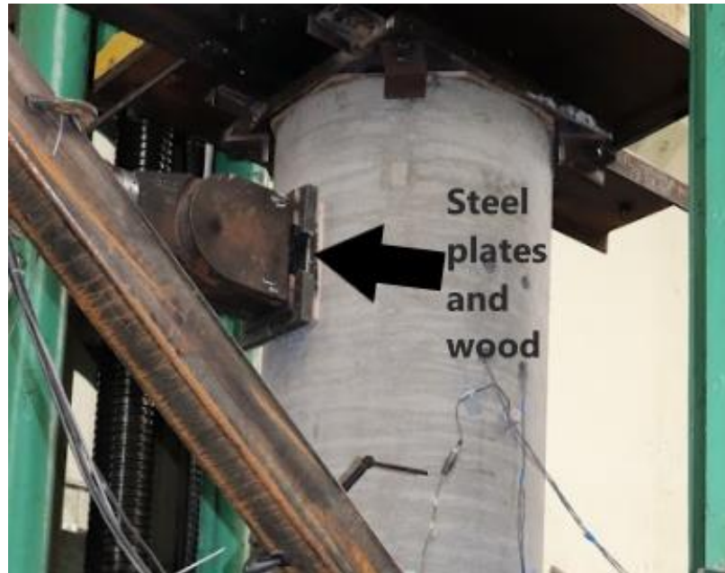
Figure 8-4. Packing underneath actuator connected to specimen
