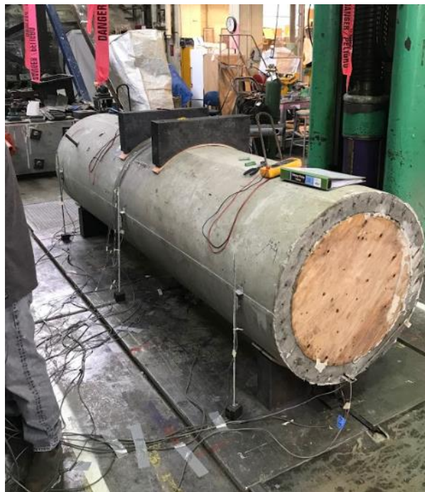
Figure 3-27. East side Duncan potentiometers attached to threaded rods that are magnetized to the lab floor
