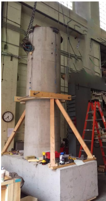
Figure 6-15. Pile-column braced on top of cap beam
