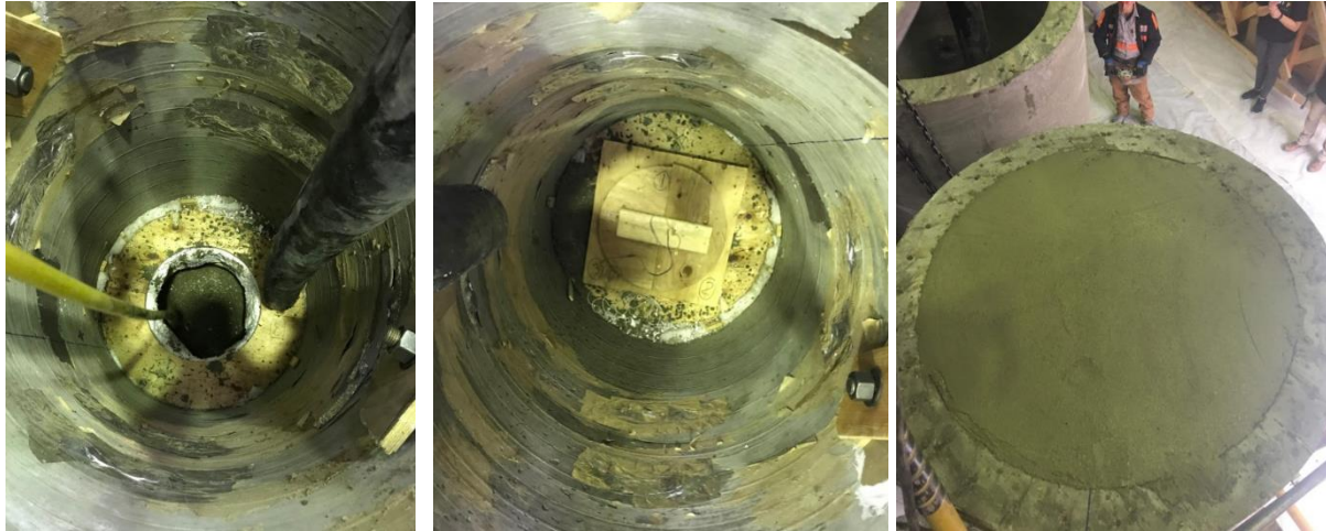
Figure 3-17. Left: Bottom half of fill concrete; Middle: Wood plug inserted; Right: Top half of fill concrete
