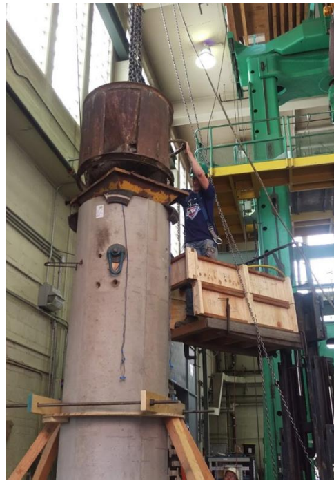
Figure 6-16. Casting plug inside of pile-column
