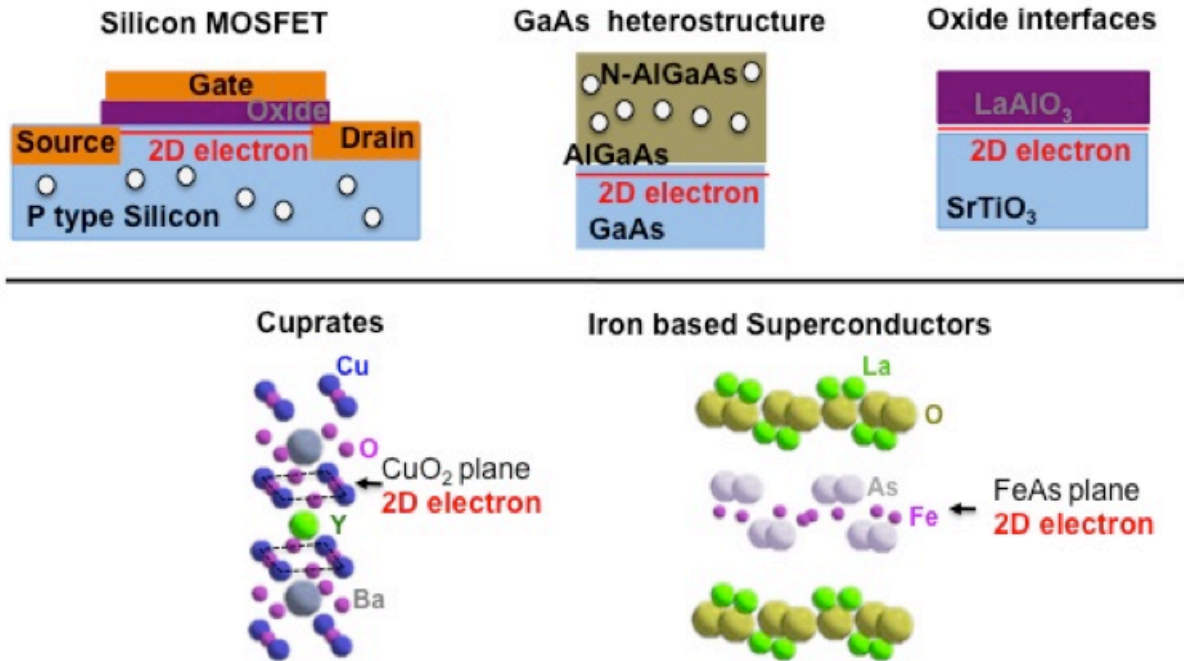
Figure 1.1. Conventional material systems hosting 2D electrons. Upper panel: 2D electronic systems induced at heterojunctions of 3D bulk materials, exhibiting QHE and superconductivity. Lower panel: typical 2D electronic systems naturally formed in layered compounds, exhibiting High-T c superconductivity.
