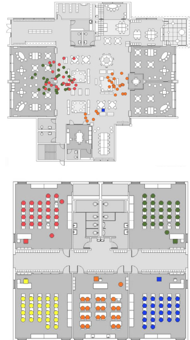
Figure 20 - Conceptual floor plan (above) compared to a traditional school floor plan (below). Credit: Parkhill, Smith and Cooper.
