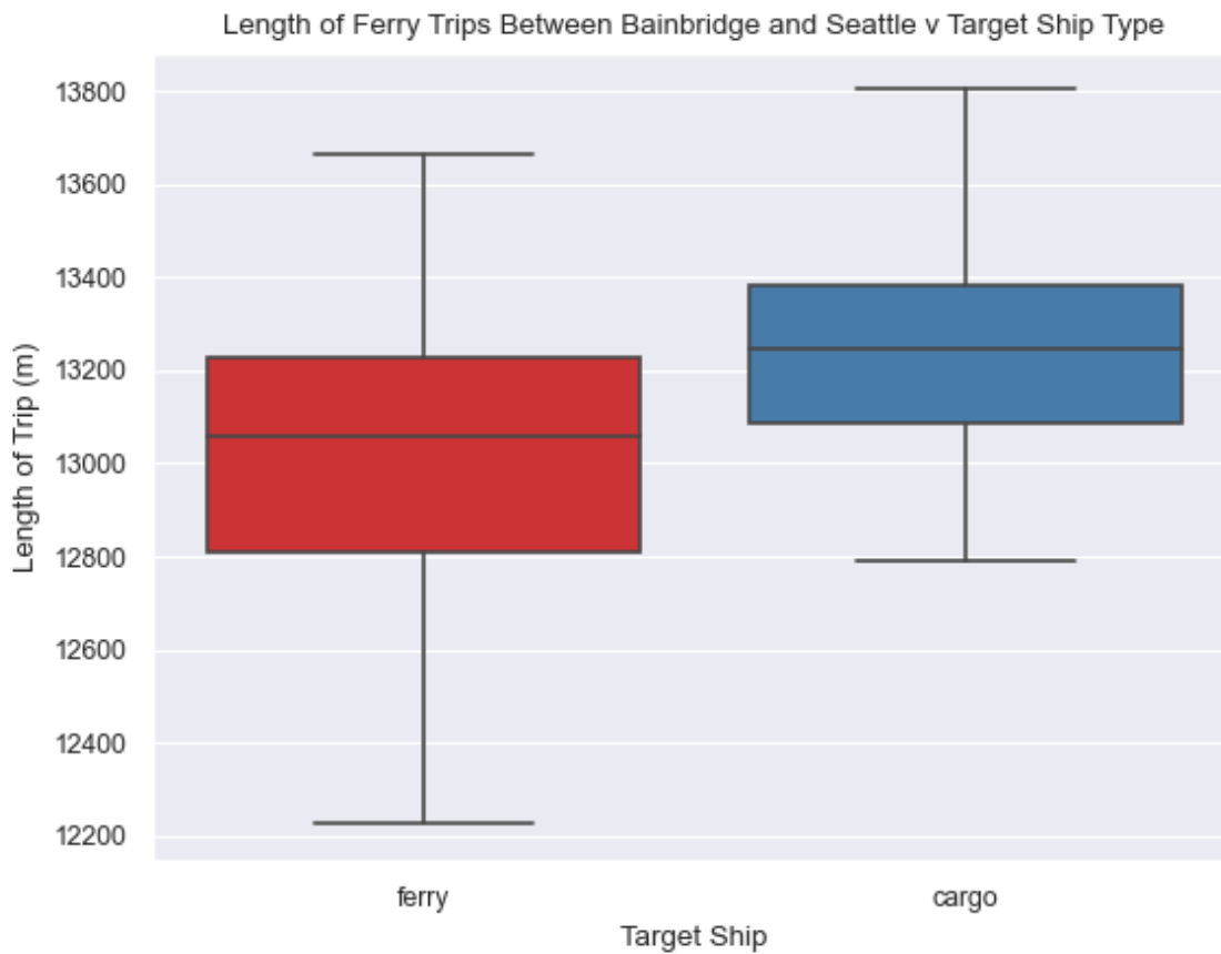
Figure 6.5: When a ferry is interacting with a cargo vessel, its route between Seattle and Bainbridge becomes lengthier.
