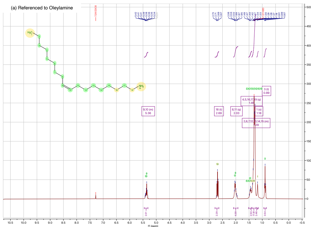
Figure 2.17. ^1\text{H} NMR (300 MHz, \text{CDCl}_3 ) \delta 5.45 – 5.31 (m, 1H), 2.69 (t, J = 6.9 Hz, 1H), 2.03 (q, J = 6.4 Hz, 2H), 1.45 (q, J = 6.8 Hz, 1H), 1.39 – 1.24 (m, 8H), 1.18 (s, 1H), 0.89 (t, J = 6.4 Hz, 2H).). Same spectra of OLA (20 mg/mL \text{CDCl}_3 ) is referenced against the chemical structure of OLA.
