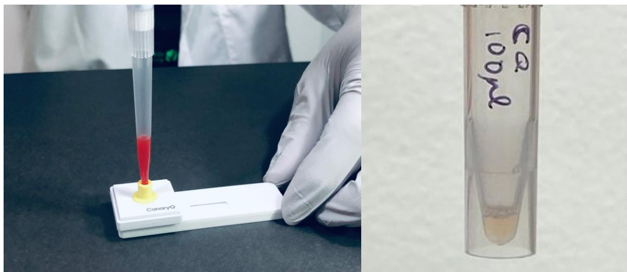
Figure 46. Left image: Image from CanaryQ depicting the use of the device. 167 Right image: Extracted plasma obtained from adding 100 \mu L of whole blood into the CanaryQ device.
