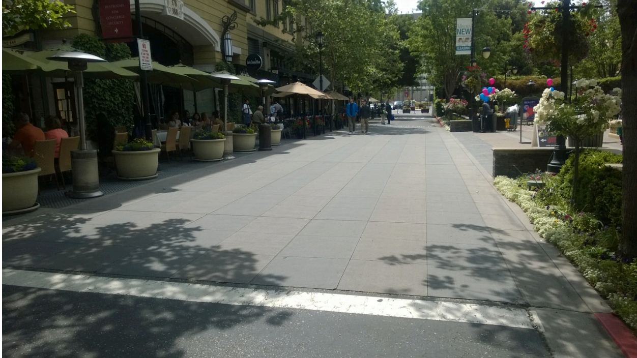
Figure 28. A long stretch of at-grade roadway with uniform paving represents shared space principles
