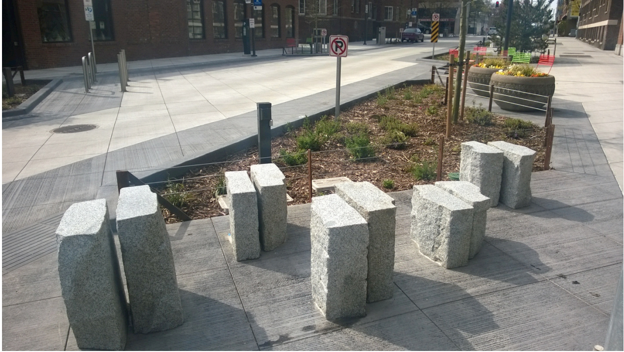
Figure 10. Small stone blocks provide secondary seating while also protecting pedestrians from the travel way
