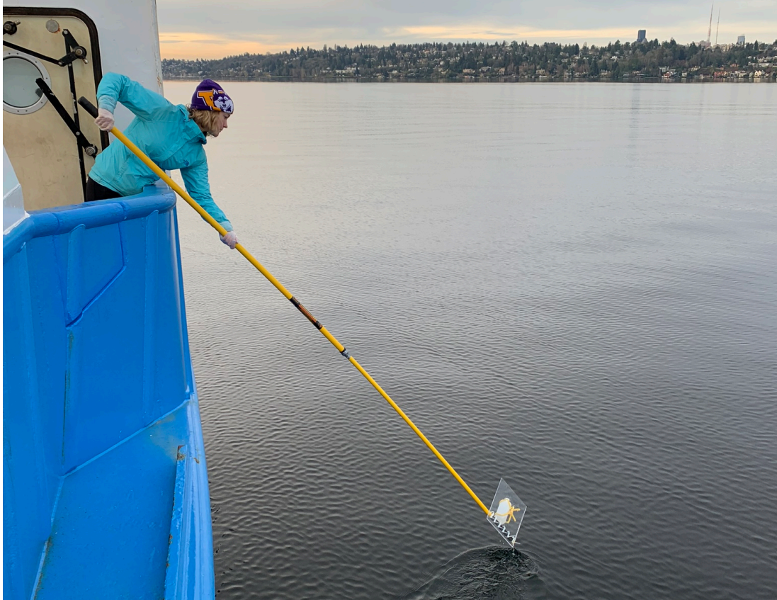
Fig. 3. Pole sampler in use to collect surface seawater samples from the R/V Rachel Carson . Photo by Julian Sachs.
