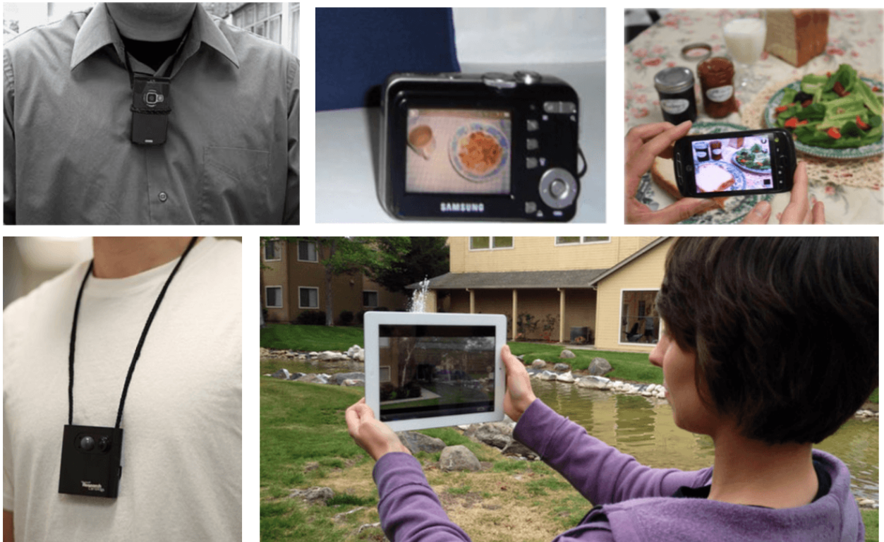
Figure 2.2: (clockwise from top left) Devices used for collecting images of food and beverages: mobile telephone with a camera around his or her neck [11], digital camera [32], mobile device with a camera [27], Microsoft SenseCam [20, 21], Apple iPad2 [44].
