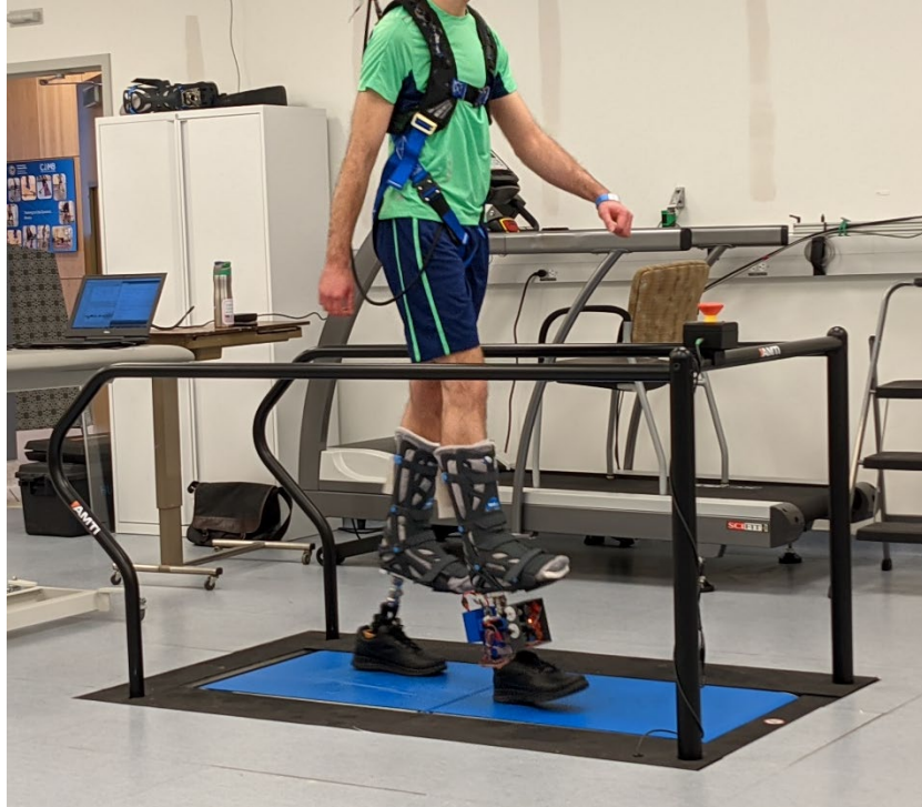
Figure 3.10 Able-bodied walking over a treadmill on the TAP device with custom boots.
