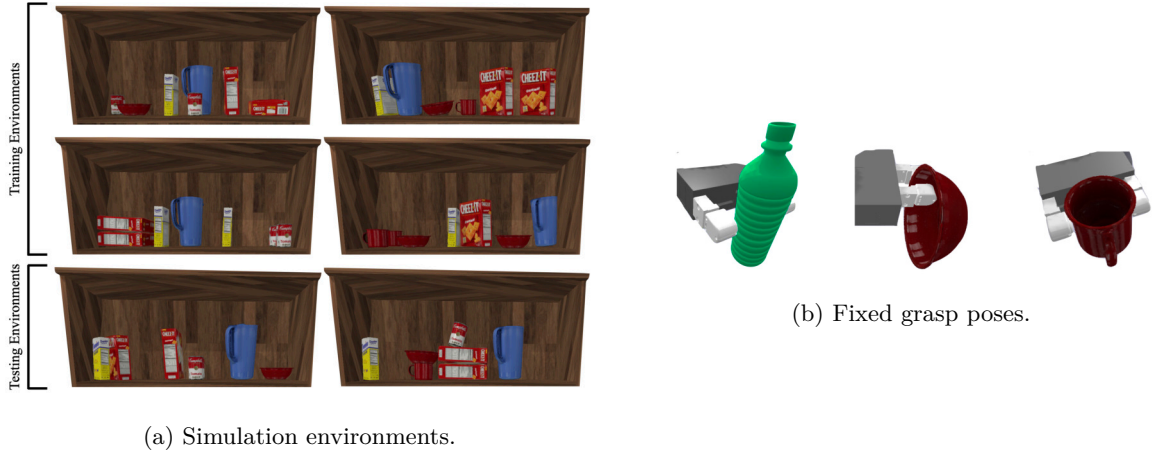
Figure 2.3: For collecting our Extrinsic Contact dataset, we simulate six kitchen cabinet environments (left) and utilize fixed, rigid grasp poses for all bottles, bowls, and mugs (right). Objects in these environments can move as the robot interacts with them during data collection.
