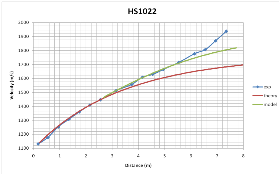
Fig. B.24 HS1022, UW, Mg-alloy, 62.76 g, 24 atm
