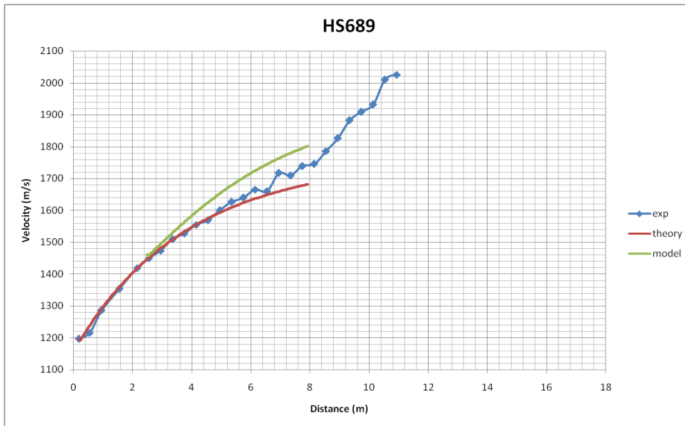
Fig. B.6 HS689, UW, Mg-alloy, 66.38 g, 23 atm
