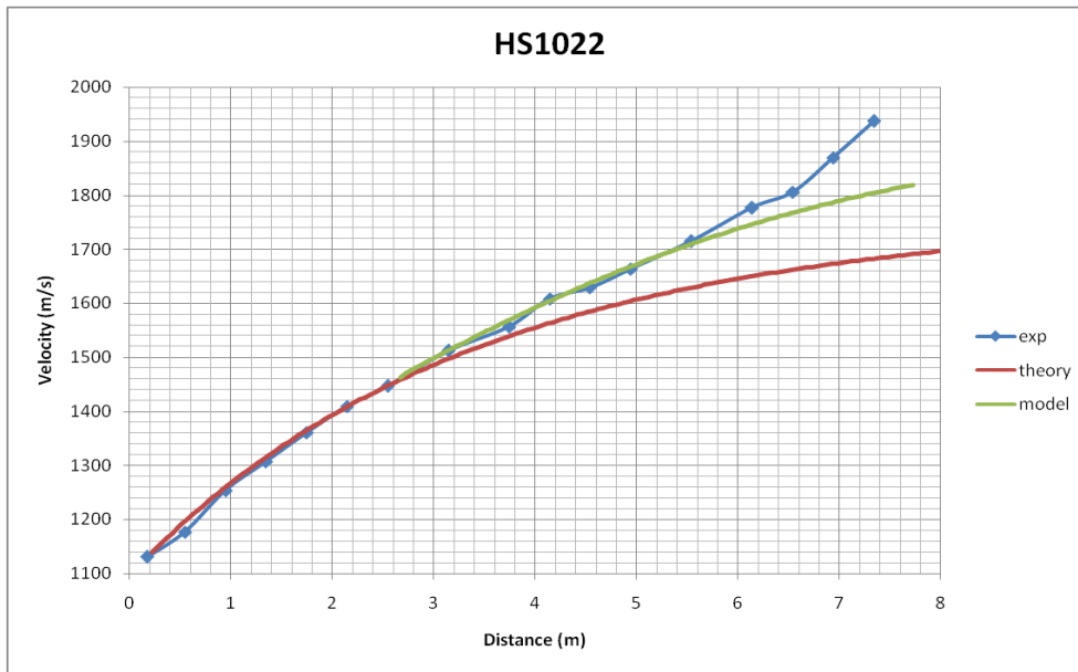
Fig. 4.15 HS1022, UW, Mg-alloy, 62.76 g, 24 atm
