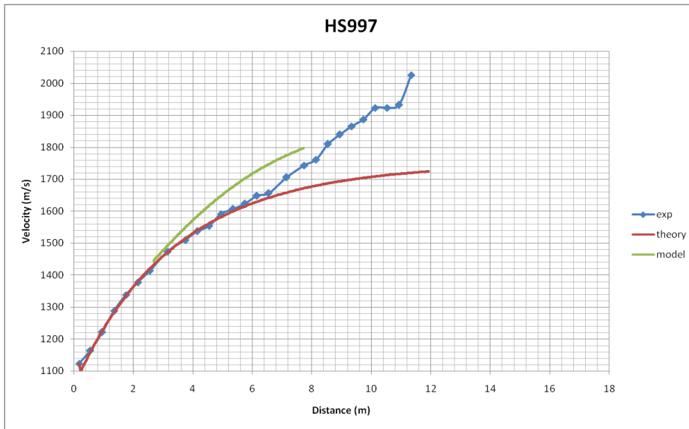
Fig. B.16 HS997, UW, Mg-alloy, 63.3 g, 23 atm
