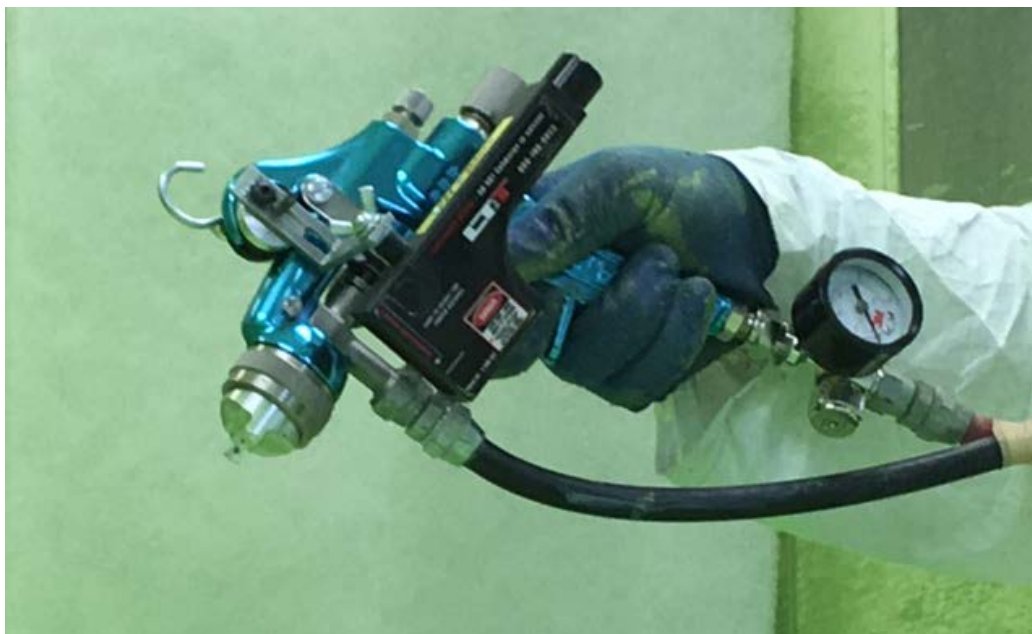
Figure 3. High Volume Low Pressure (HVLP) Spray Paint Gun (blue) with Laser Guide (black)
