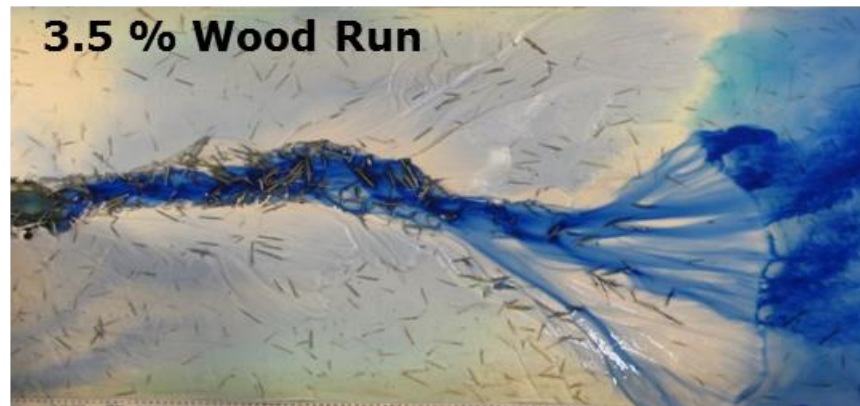
Fig. 10 Overhead photos during the 2 nd hold period showing increased bifurcations and multiple simultaneously occupied channels on the delta for the experimental runs with exhumed wood debris. Experimental runs with exhumed wood show more pools, more logjam complexity, more topographic depth variability, more channel edge lengths and more delta shoreline length.
