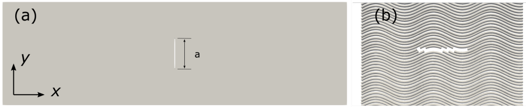
Figure 7.5: Specimen for fracture simulations: (a) CCT specimen modeled in DM4C; (b) Magnified view of an example of wavy reinforcement near the crack.
