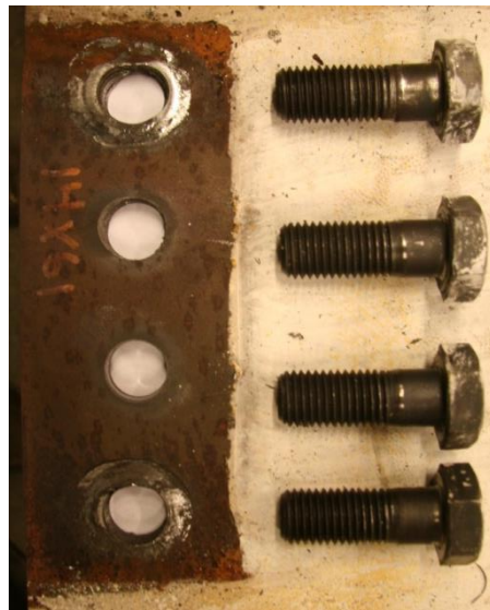
Figure 4.56: S beam web bolt hole elongation.
