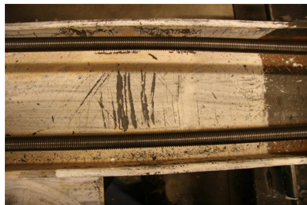
Figure 4.17: Initial local buckling in N (left) and S (right) column flanges at +2.2\% drift (LB1-OF/IF).
