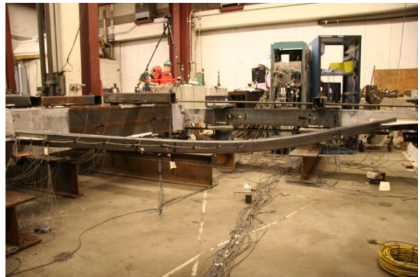
Figure 4.7: N brace buckling at +0.7% drift (B1).
