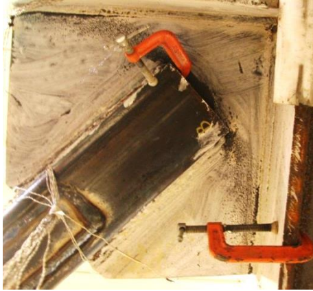
Figure 4.41: GP yielding at 1.7% drift (Y1).
