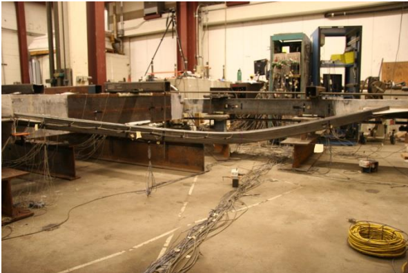
Figure 4.9: N brace buckling at +1.1\% drift (B2).
