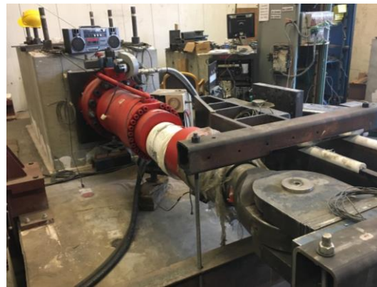
Figure 3.3: Hydraulic actuator and reaction block.
