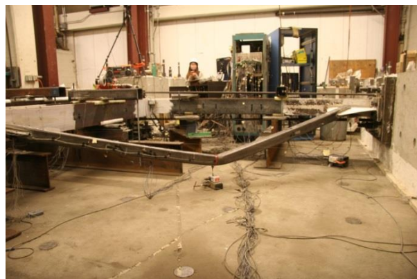
Figure 4.53: N brace buckling at 3.3% drift (B3-PH).
