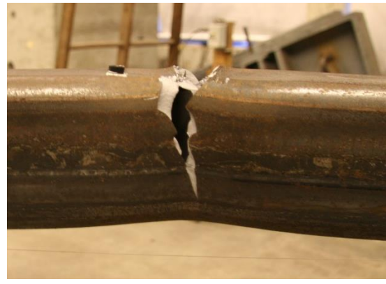
Figure 4.85: S brace \frac{3}{4} tear at 3.6% drift (B3-BT).
