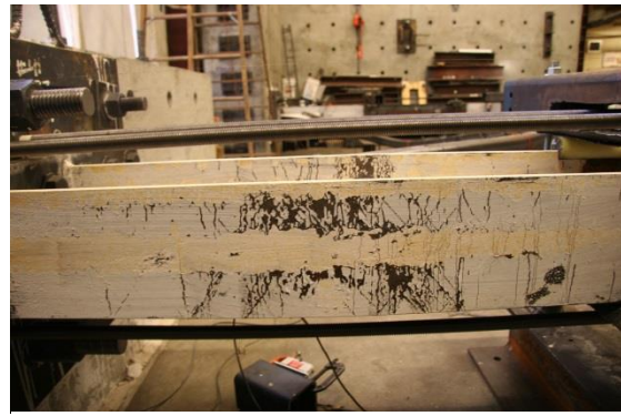
Figure 4.44: N col. moderate yielding at 1.9% drift (Y1-OF/IF).
