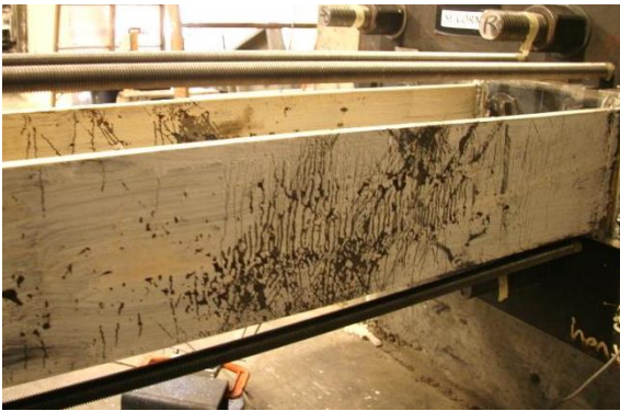
Figure 4.43: S col. moderate yielding at 1.9% drift (Y1-OF/IF).
