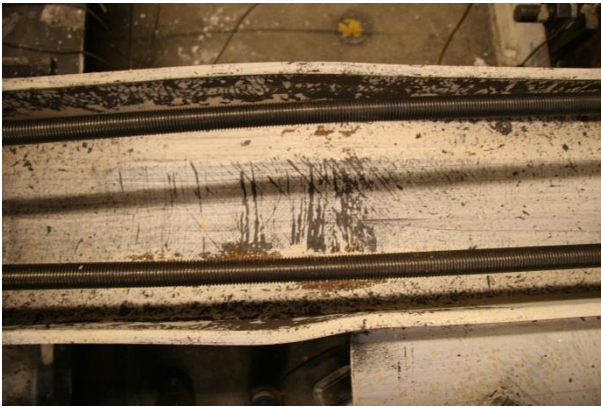
Figure 4.84: N col. moderate local buckling at -3.3% drift (LB2-OF/IF).
