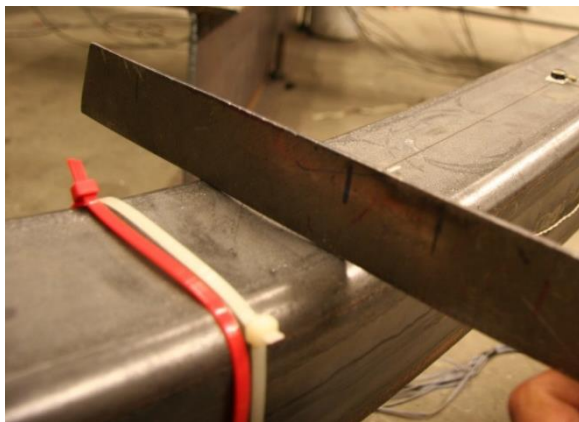
Figure 4.15: S brace initial cupping at -1.9% drift (B3-PH).
