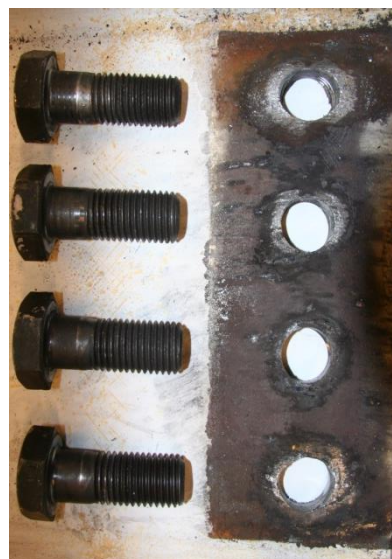
Figure 4.57: N beam web bolt hole elongation.
