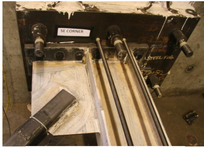
Figure 3.8: Base plate attached to interface plate.
