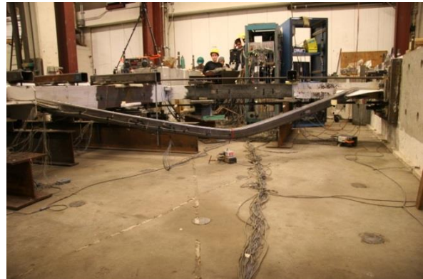
Figure 4.46: Brace buckling at 2.5% drift (B1).
