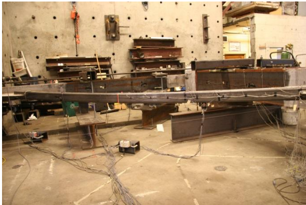
Figure 4.6: S brace buckling at -0.28% drift (B1).
