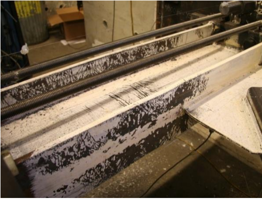
Figure 4.76: N col. severe yielding at 2.8% drift (Y3-PH).
