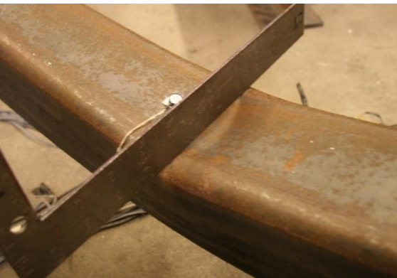
Figure 4.78: S brace cupping at 3.0% drift (B3-PH).
