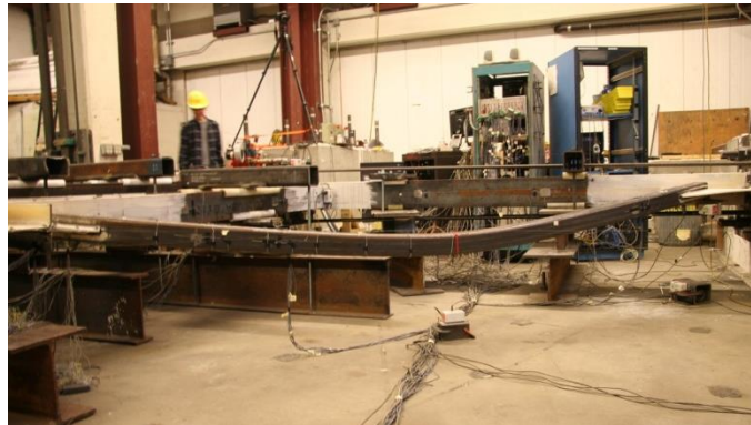
Figure 4.67: N brace buckling at +0.83% drift (B2).
