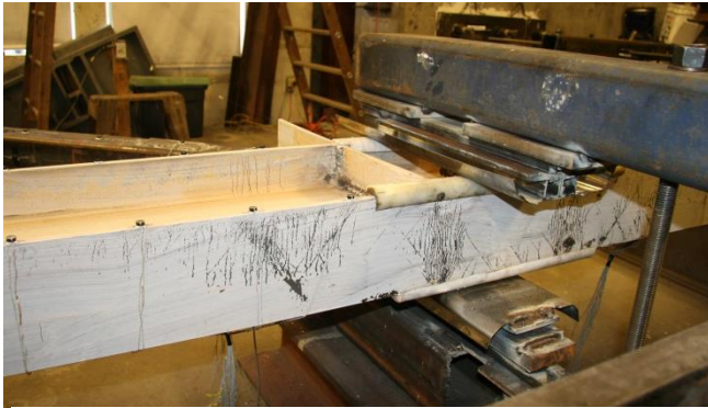
Figure 4.72: Beam OF yielding at 1.9% drift (Y1-OF).
