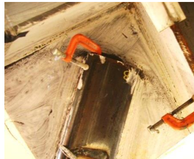
Figure 4.36: Mid-span GP yielding at -0.83% drift.
