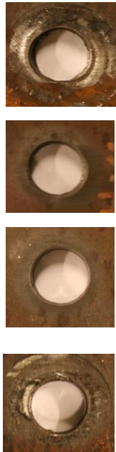
Figure 4.56: S beam web bolt hole elongation.
