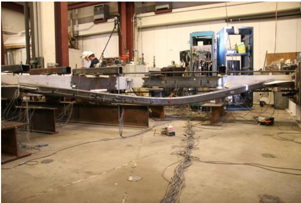
Figure 4.37: N brace buckling at +1.1\% drift (B1).
