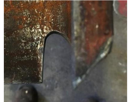
Figure 3.25: Completed weld access hole.
