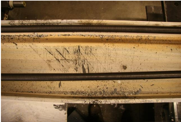
Figure 4.45: Initial col. local buckling at 2.2% drift (LB1-OF/IF).
