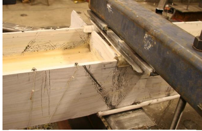
Figure 4.55: Extent of beam yielding at end of test (Y1-OF/IF).
