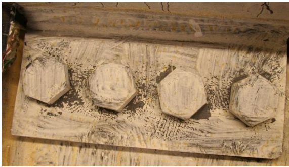
Figure 4.86: Shear tab moderate yielding at +3.3% drift (Y2).
