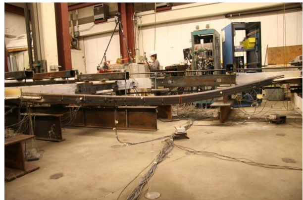
Figure 4.62: N brace buckling at 0.7% drift (B1).
