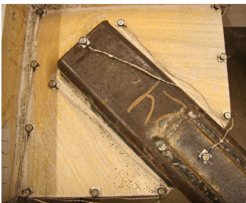
Figure 4.63: Mid-span GP initial yielding at 0.4% drift (Y1).
