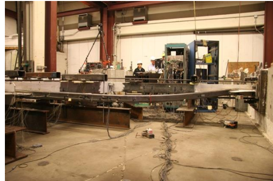
Figure 4.34: N brace buckling at 0.41% drift (Y1).
