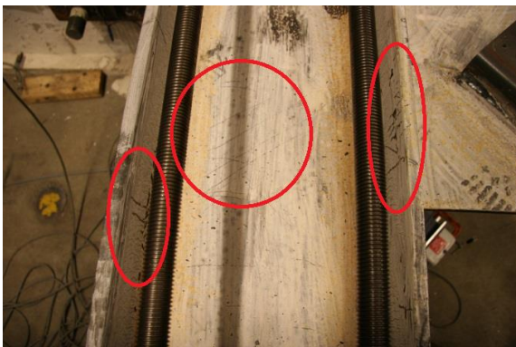
Figure 4.11: N col. initial yielding at +1.4\% drift (Y1).
