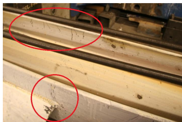
Figure 4.40: S col. initial yielding at +1.4\% drift (Y1-OF).
