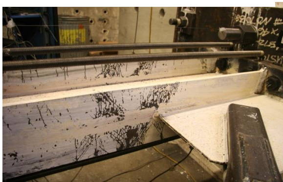
Figure 4.70: N col. moderate yielding at 1.9% drift (Y2-PH).
