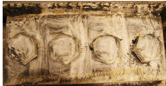
Figure 4.66: S shear tab yielding at -0.83% drift (Y1).
