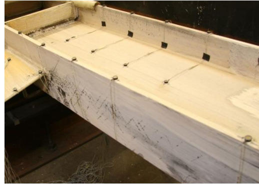
Figure 4.73: Beam IF yielding at 1.9% drift (Y1-OF).
