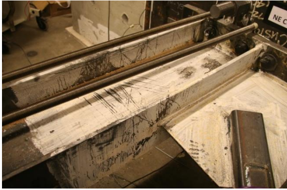
Figure 4.13: N col. moderate yielding at +1.9% drift (Y2-PH).
