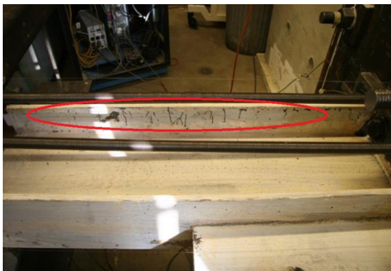
Figure 4.39: N col. initial yielding at +1.4\% drift (Y1-OF).
