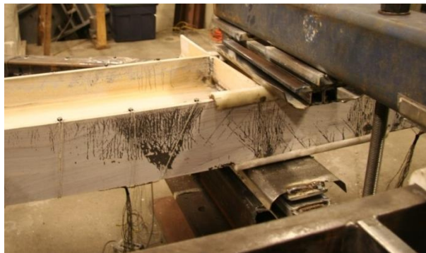
Figure 4.87: Beam top flange moderate yielding at +3.3% drift (Y3-OF).
