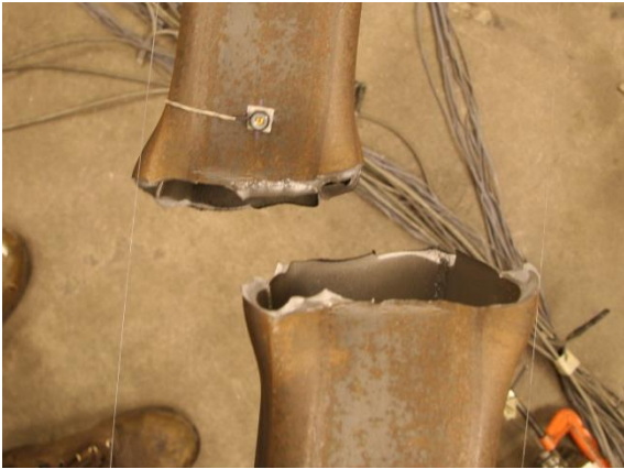
Figure 4.88: N brace fracture at -3.6% drift (B4-BF).
