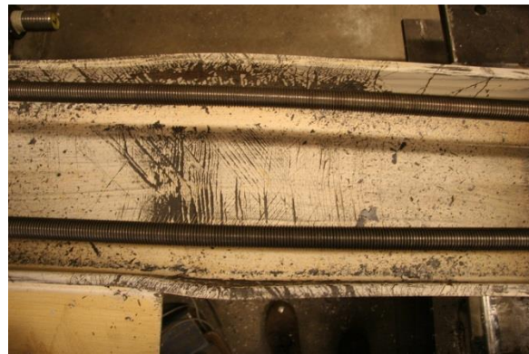
Figure 4.79: S col. moderate local buckling 3.0% drift (LB2-OF/IF).
