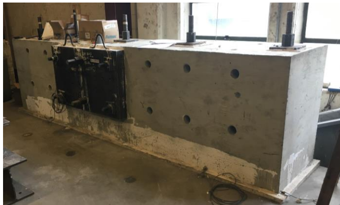
Figure 3.2: Reaction block used for N column anchorage.
