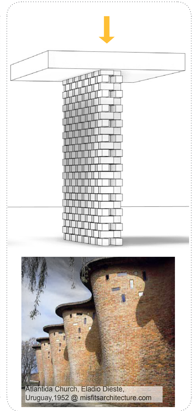
Figure 20: Multiple-wythe brick wall
