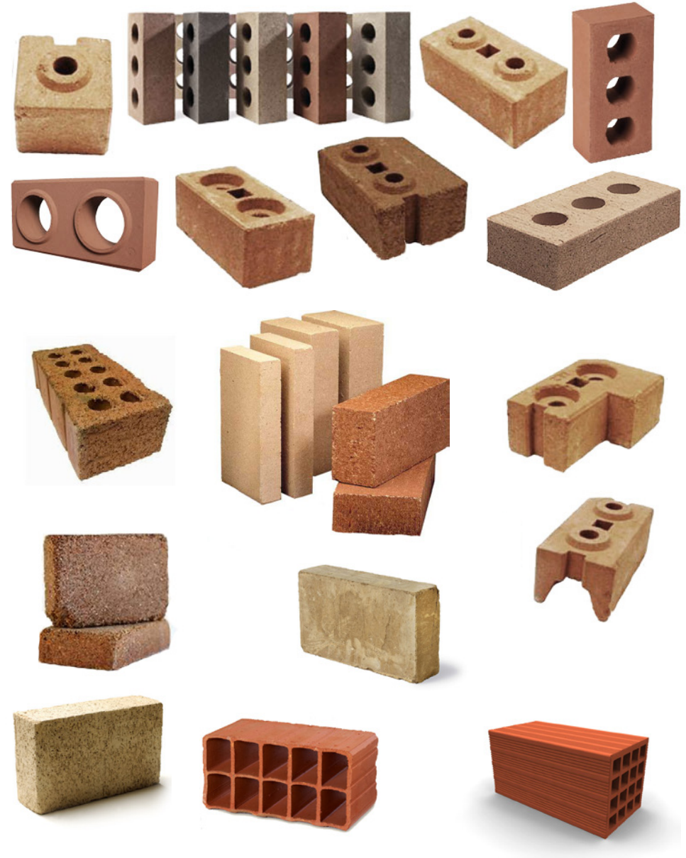
Figure 8: Bricks including fired bricks, mud bricks and CEBs
