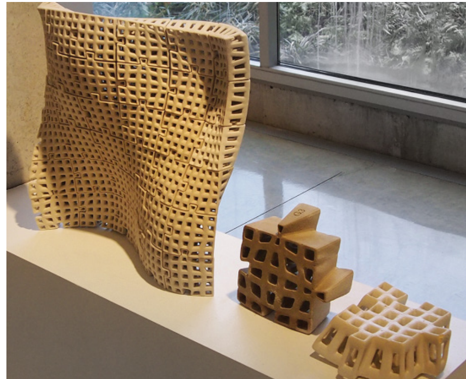
Figure 29: 3D printed bricks, http://www.news.cornell.edu/stories/2014/07/3-d-printing-helps-designers-build-better-brick .
