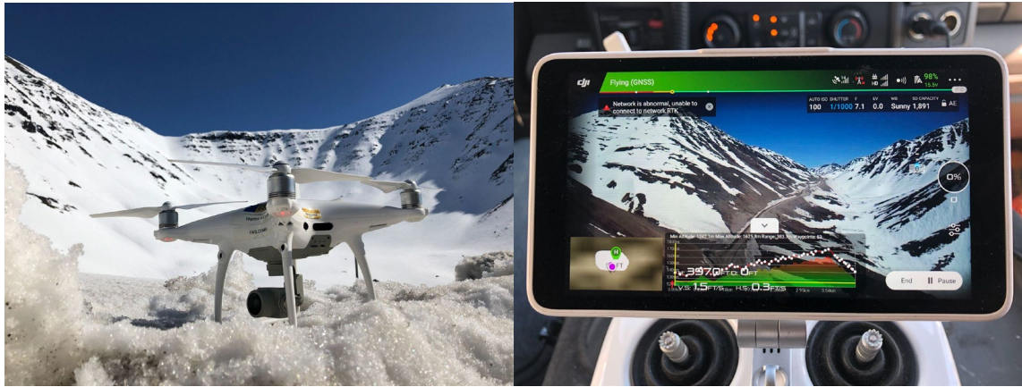
Figure 3.5 DJI Phantom 4 RTK (a) and DJI controller (b) being used in Atigun Pass, Alaska
