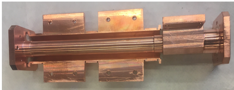
Figure 3.15: Photo of the thin walled decay cell (13 mil wall thickness) built in order to overcome the eddy current issue. One can see the step down to the thinner walls in the central region of the cell.
