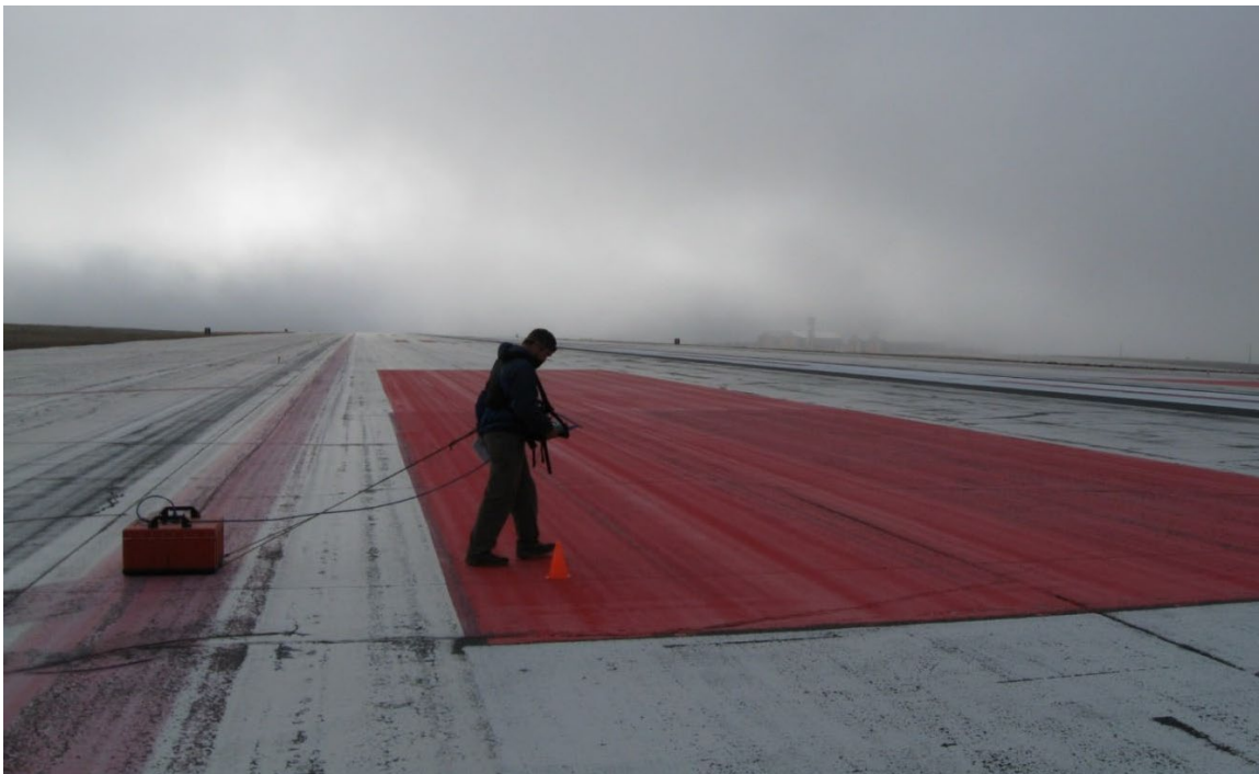
Figure 3-7 200-MHz antenna pulled over an airfield embankment.
