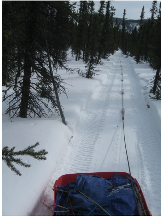
Figure 3-4 CCR system pulled by a snowmobile on a packed trail
