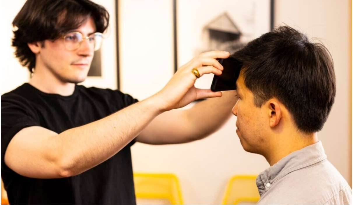
Figure 3.1: A demonstration of the physical interaction used to test an individual’s core body temperature by bringing the smartphone screen in contact with the user’s forehead. This interaction allows for the smartphone screen to measure the amount of contact which influences heat exchange which is measured by the device’s internal thermistors.
