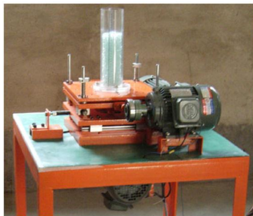
Figure 2.14: Setup used for packing large spheres by Li et al [32]
