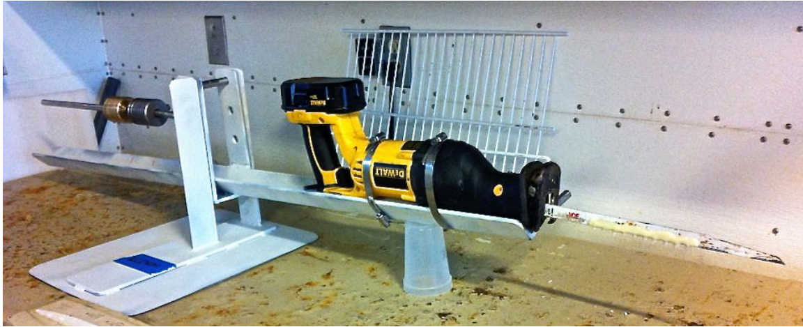
Figure 1 , Setup for DeWalt 385 reciprocating saw. Weight placed on posterior allows consistent drop and force on blade. Built by Jeff Brash, 2014.
