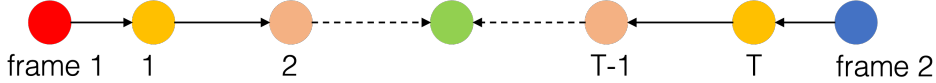
Figure 4.5: Recursive synthesis. To fill in a jump cut with smooth, intermediate frames, we recursively fill in frames from the end towards the middle.
