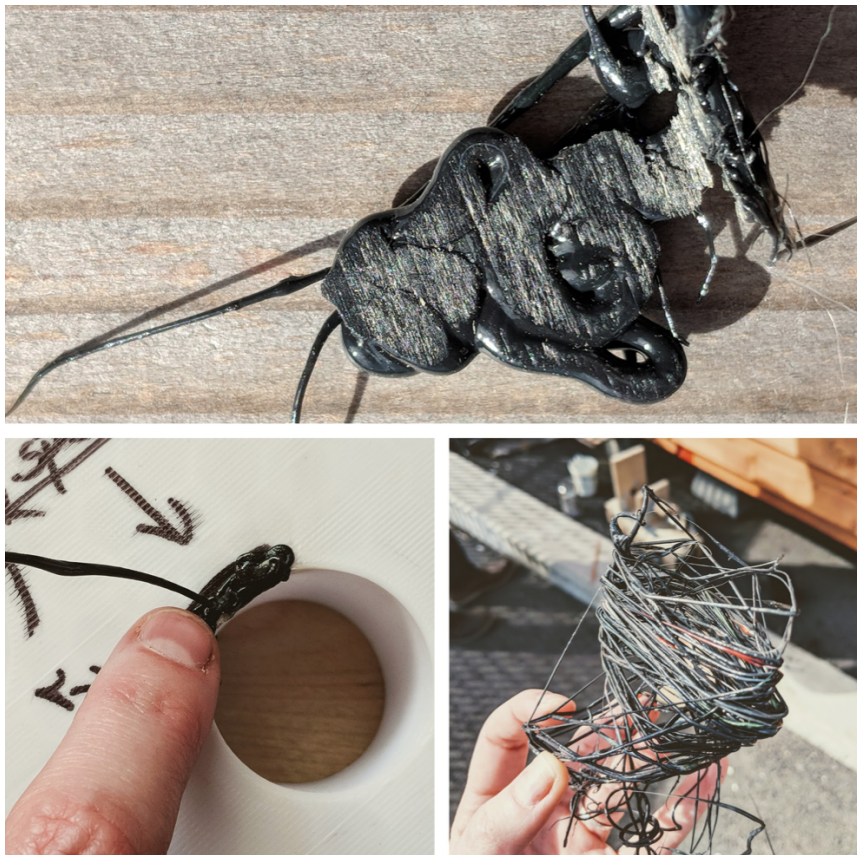
Figure 2: Molding forms and textures, patching failed prints, and spinning forms with discarded PLA filament.
