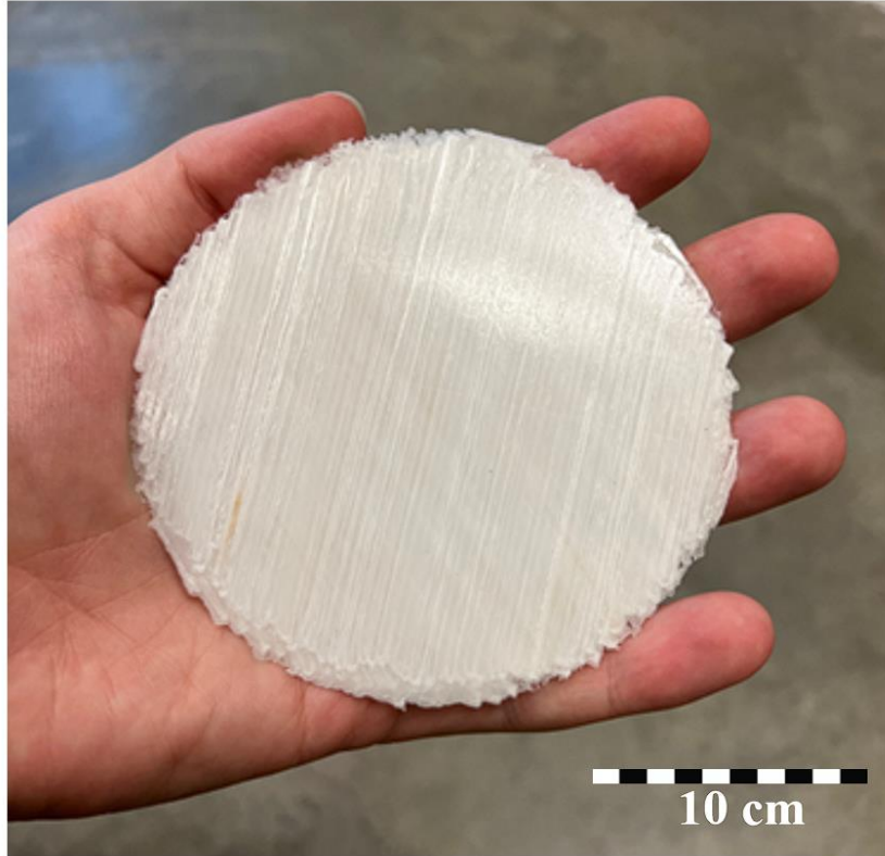
Figure 3.4. A printed Dyneema/PCL composite disk with a bouligand structure
