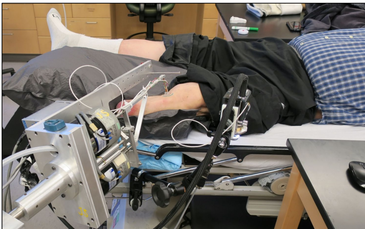
Figure 3.24. Load application during the RH Test. Participants laid supine on a hospital bed. As shown here, the Biaxial Load Applicator was often rotated so that the load applicator pad matched the angle of the skin's surface, thus reducing pressure concentrations on the edges of the pad.
