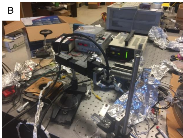
Figure 4-6. Schematic (A) and Picture (B) of the impact test. A closeup of the sensor on an aluminum beam shows the laser doppler vibrometer over the IDEs (C).
