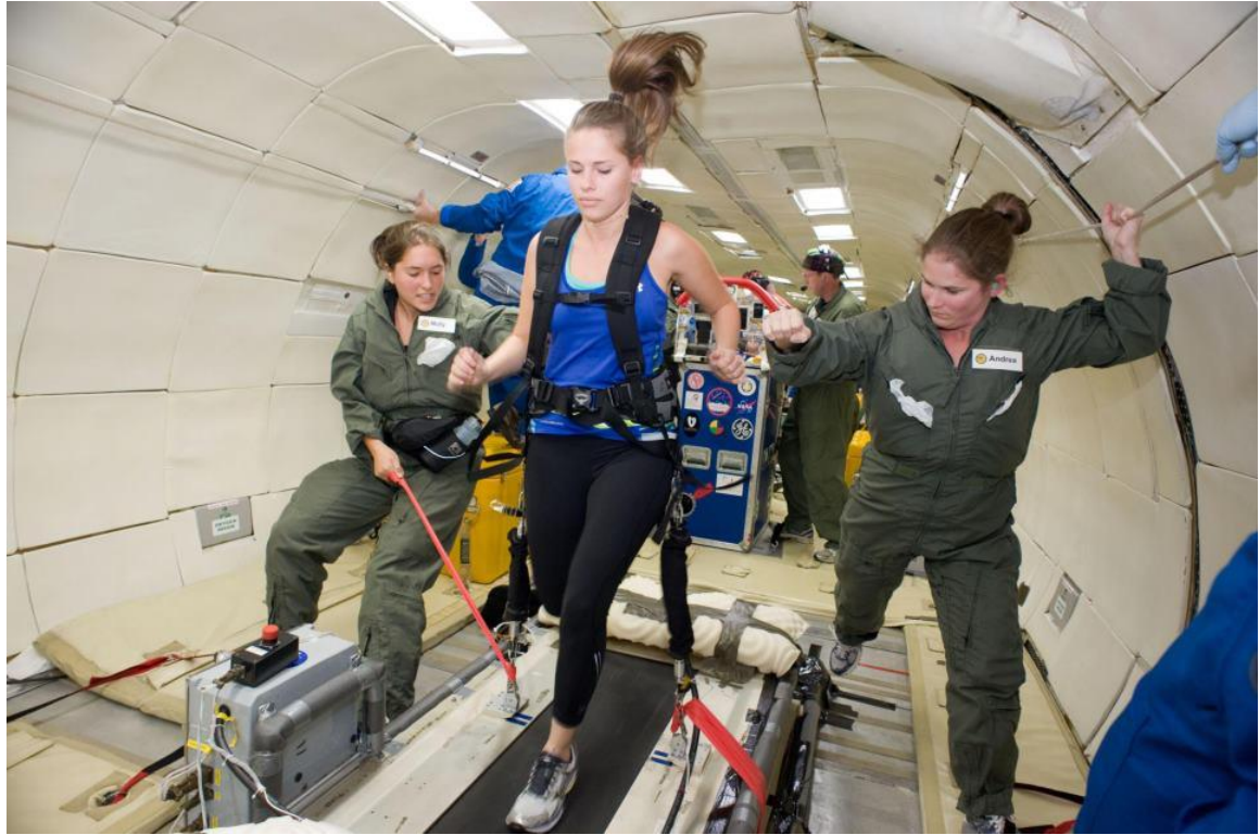
Figure 9 Subject running on a treadmill in zero gravity with a 1 body weight (1 BW) load applied via the C-SLD and harness system during a parabolic flight
