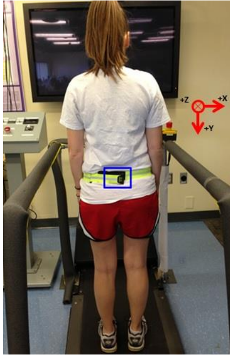
Figure 11 Subject shown on treadmill wearing accelerometer in the mid-lower back; orientation of the sensor axes for both the 1g and parabolic flight are shown to the right of the subject in red
