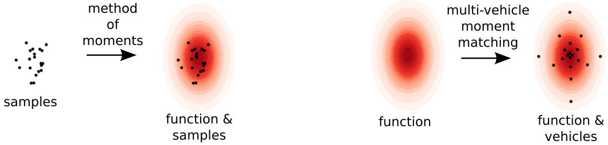
Figure 3.1: An illustration of the method of moments and multi-vehicle moment matching formulation with a 2-d function. The statistical method of moments (left) determines parameters of a function based on samples. The multi-vehicle moment matching idea in this thesis (right) determines vehicle positions based on a function.
