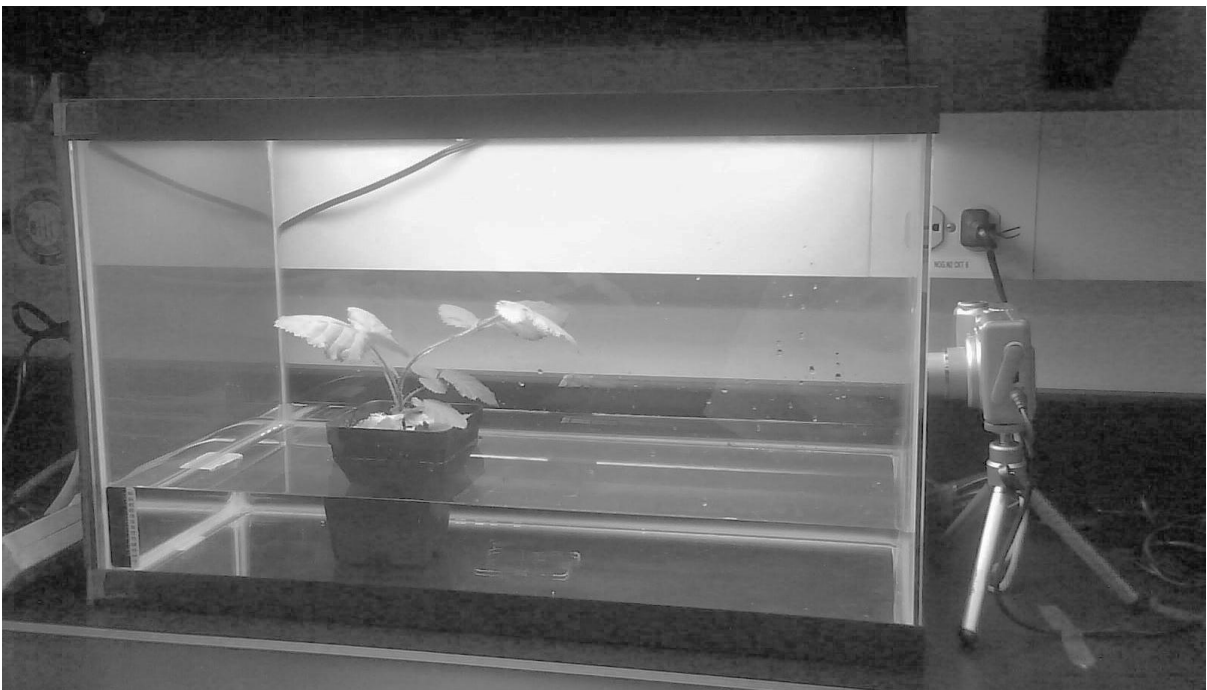
Figure 8. Partially-filled submergence tank and time-lapse camera at the start of a submergence trial. The tank was completely filled during the experiment.
