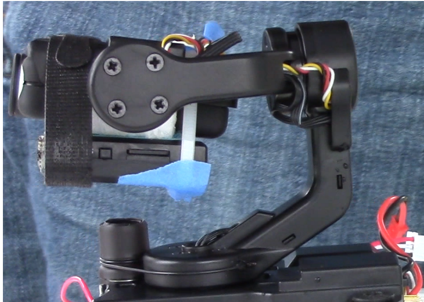
Figure 2.7: Gimbal yaw potentiometer setup.
