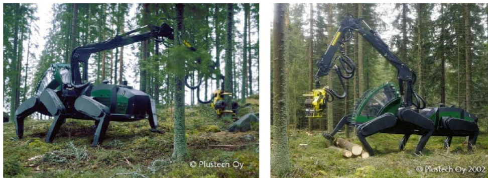
Figure 29. John Deere Walking Forest Harvester 69
