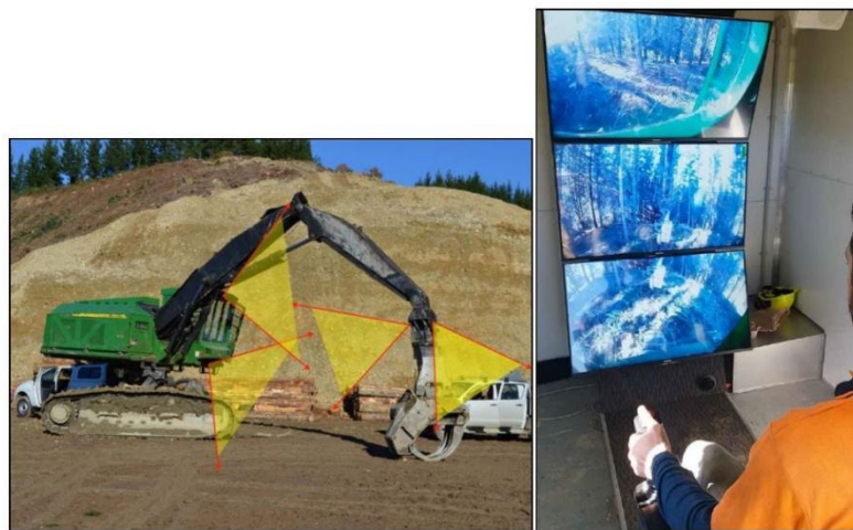
Figure 25. Camera Locations and Remote Control Apparatus 65
