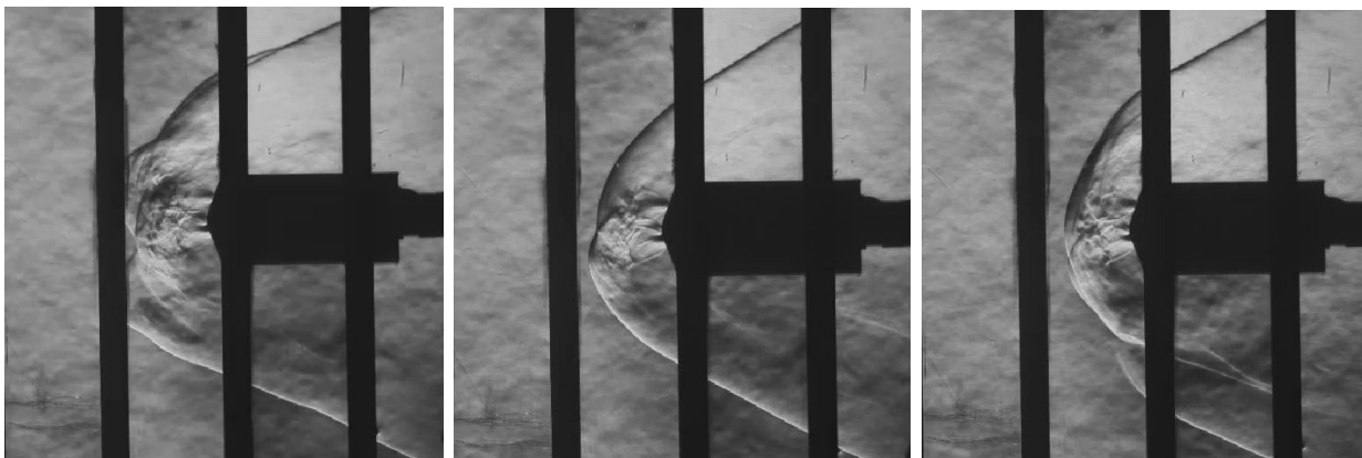
Figure 5.5: Frames from an Oscillating Case with Penetration: Quad Nozzle, Mach 3, C_T=1 , \alpha=0^\circ .
