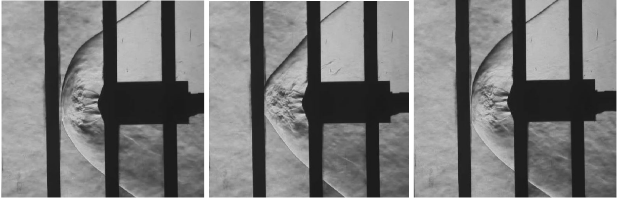
Figure 5.2: Frames from an Oscillating Run, Quad Nozzle, Mach 2, C_t=1 , \alpha=0^\circ .
