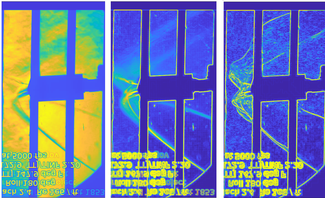
Figure 3.9: Example of feature extraction from SRP data from LaRC at Mach 2, tri-nozzle at 4^\circ angle of attack from Berry[10]. From left to right: mean schlieren field, mean field of gradient magnitude, instantaneous gradient magnitude field.
