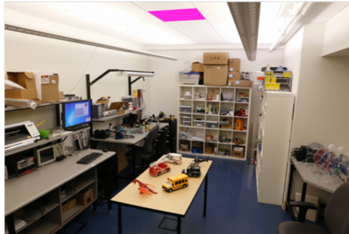
Figure 3.3: Lab environment used for initial IDSense testing. The RFID reader antenna is placed on top of a ceiling panel (highlighted in pink) pointing downwards.
