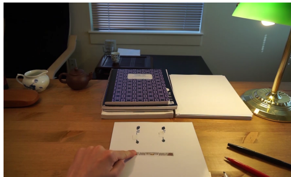
Figure 4.9: PaperID example application: light controller using a single RFID sticker
