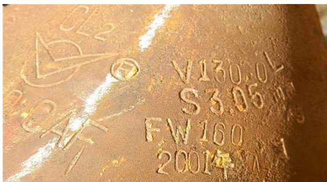
Figure 3: A chlorine gas canister clearly showed the marking of the Chinese arms manufacturer Norinco and the stamp Cl 2 , the scientific shorthand for chlorine, as well as the character 年 (Nián), meaning “year” 34
