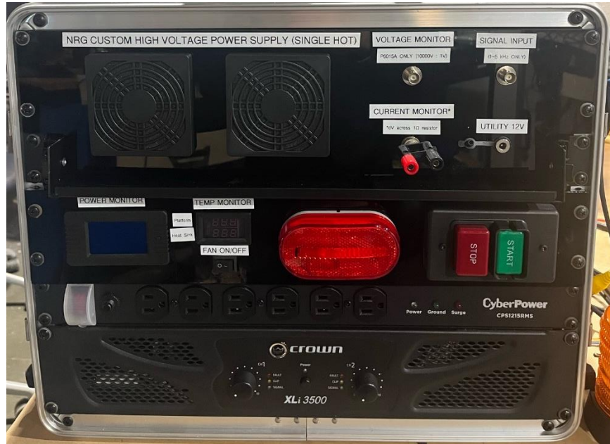
Figure 3.8. The “single hot” custom power supply is built with a power strip, amplifier, power monitor, temperature monitor, voltage monitor, current monitor, utility 12V, and signal input. The temperature monitor typically monitors the custom transformer’s core.
