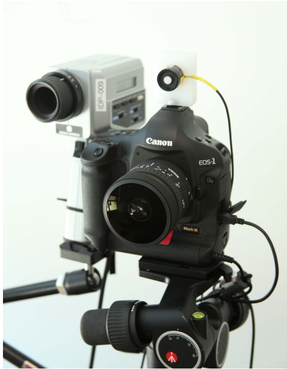
Figure 20 - Canon camera, luminance meter, Li-Cor 210sa from seated eye position
