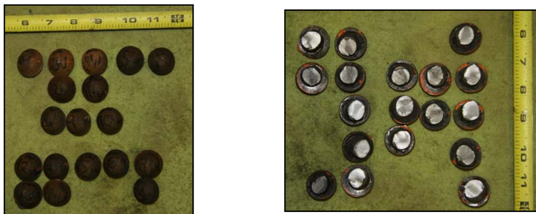
Figure 4.66 West Guardrail Fractured Rivets – Specimen 17R
