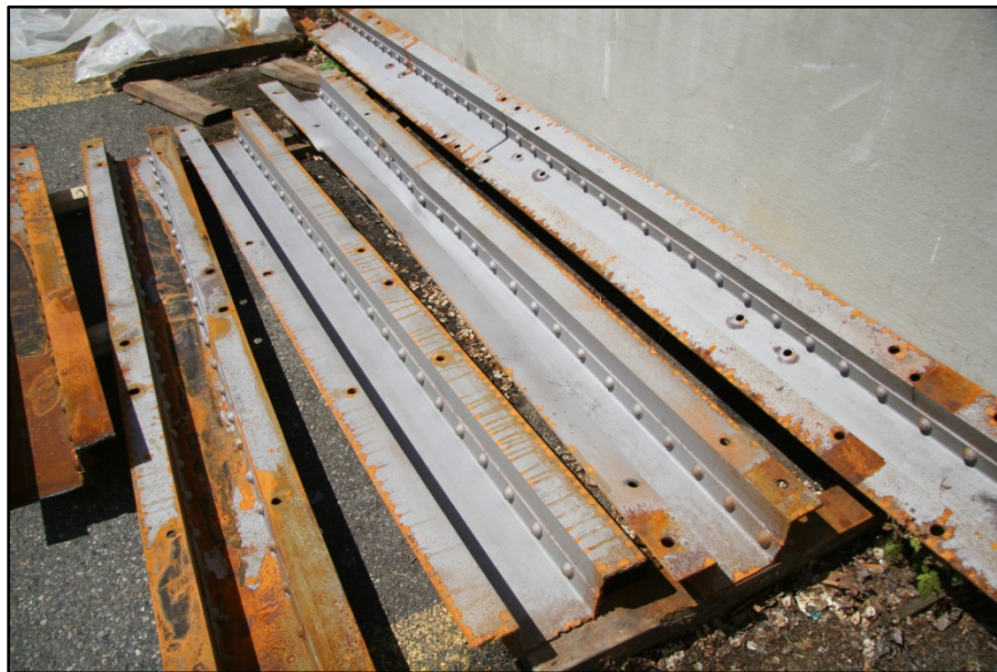
Figure 3.8 Guardrail Specimens after Sandblasting
