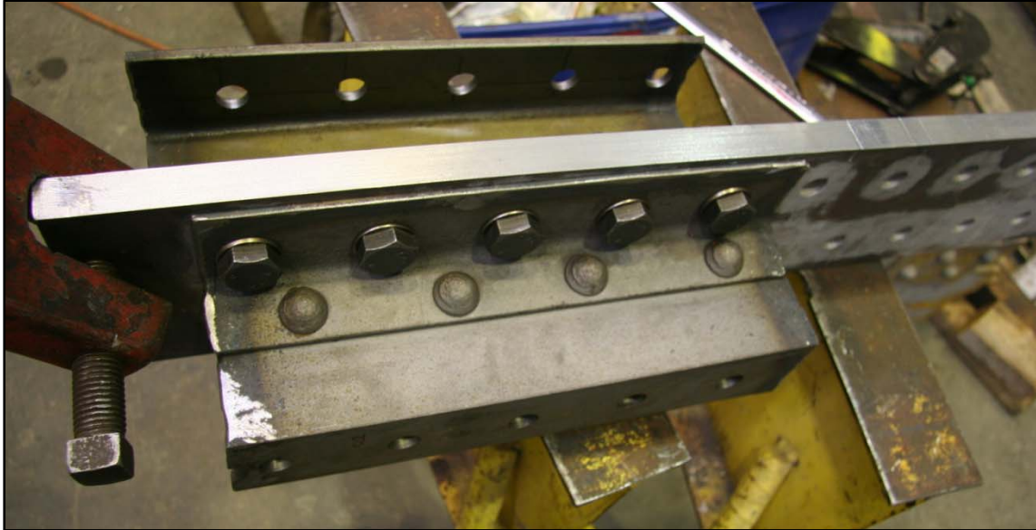
Figure 3.36 Guardrail Bolted to Middle Plate
