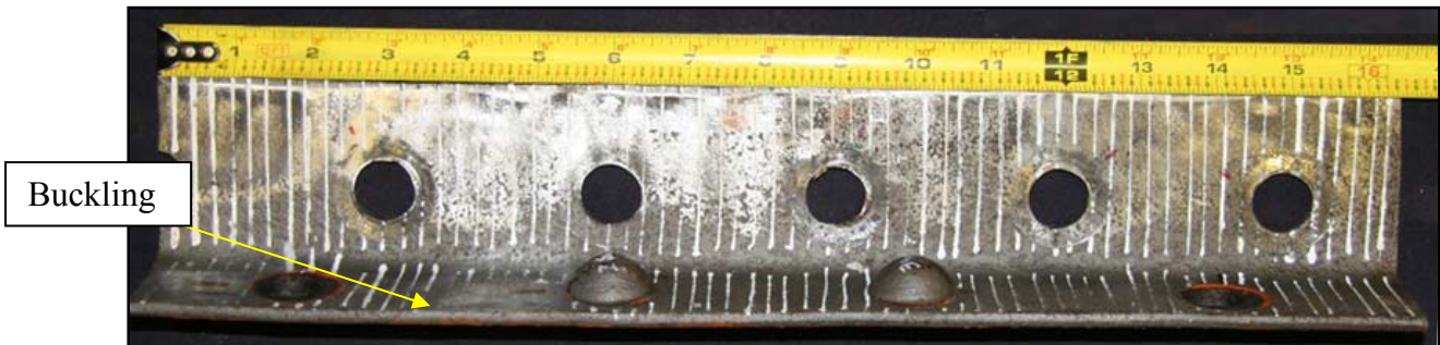
Figure 4.21 West Channel Buckling – Specimen 4R
