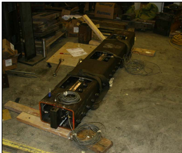
Figure 3.42 Baldwin Specimen After Attachment of Middle Plate to HSS
