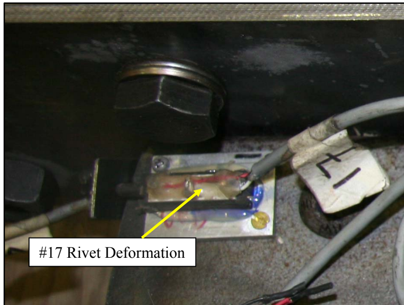
Figure 3.37 Attachment to Guardrail to Measure Rivet Deformation
