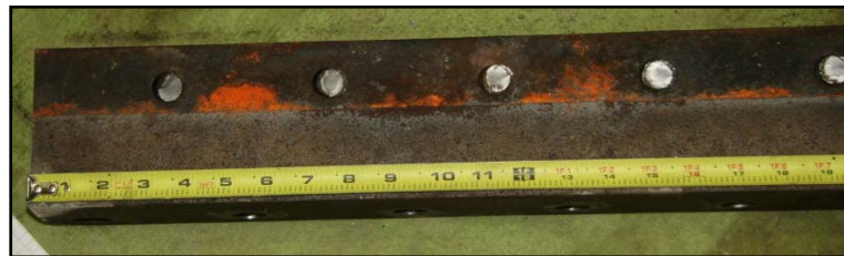
(b) Top of Angle After Testing
