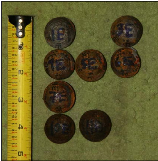
(a) (b) Figure 4.60 East Guardrail Fractured Rivets - Specimen 11R
