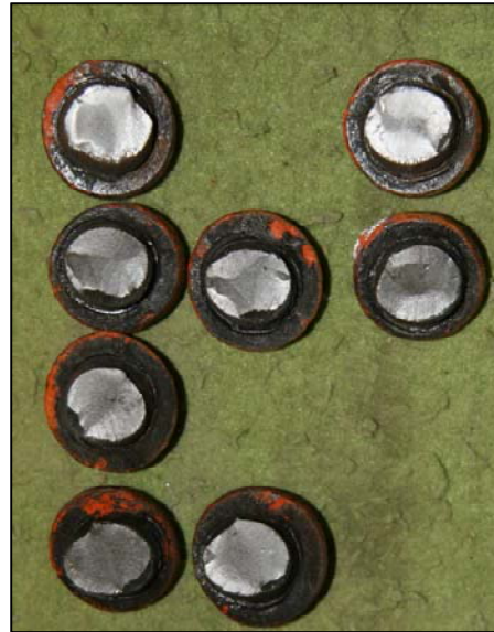
(a) (b) Figure 4.60 East Guardrail Fractured Rivets - Specimen 11R
