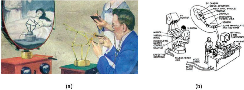
Figure 6.1: Teleoperated robotic surgery concept: (a) from Hugo Gernsback’s illustration in 1925, (b) proposed by NASA Advanced Concepts and Missions Division in 1972
